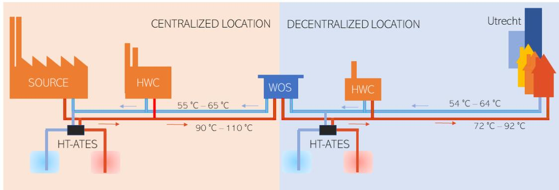
Fig. 6. Possible locations for the HT-ATES STES. At the surface, heat pumps bring the guarantee that heat can be delivered to the network (discharging phase) or to the heat storage (charging phase).
