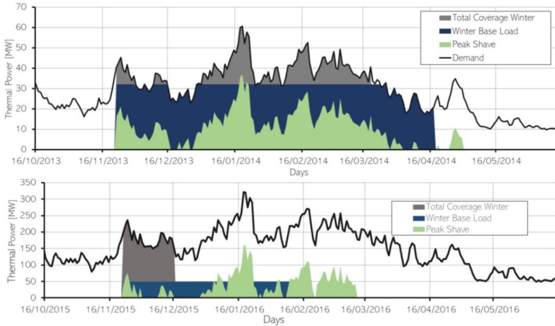
Fig. 11. Supplied thermal energy during the winter of 2015-2016 making use of an HT-ATES with 1,300,000 m<sup>3</sup> storage volume making use of different strategies: “peak shaving” (green), “winter base load” (blue) and “total winter coverage” (grey). Top: decentral location; Bottom: central location.
