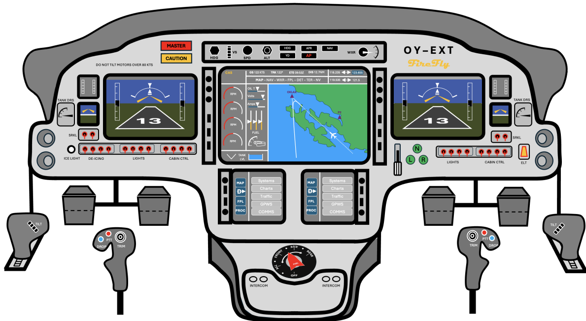
Figure 8.9: Cockpit design and layout including flight controls.
