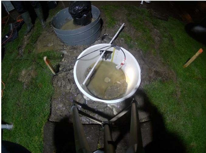
Figure 4.4: Exit point in the center of a bucket with V-notch weir.
