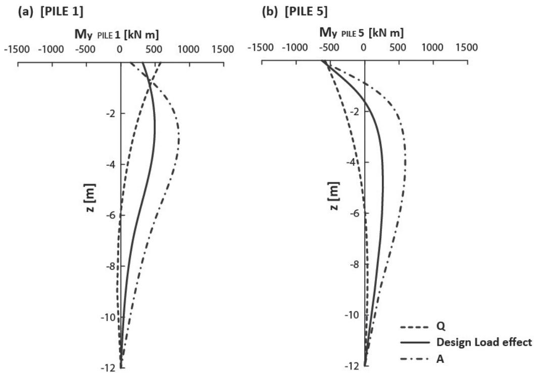
Fig. 15 – Evolution of  $M_{y\text{PILE}}$  for the most loaded piles ( $P1=P6$  and  $P5=P7$ ).
