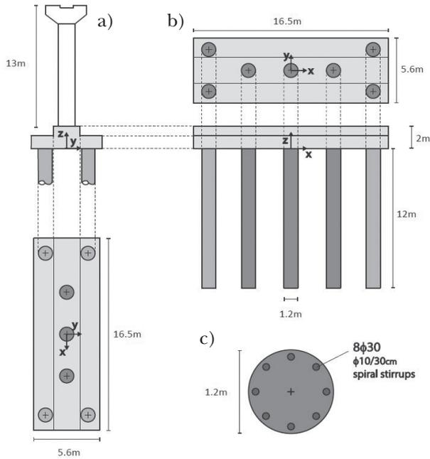
Fig. 3 – Geometry of the piled raft foundation: a) transversal section; b) longitudinal section; c) cross section of the single pile.
