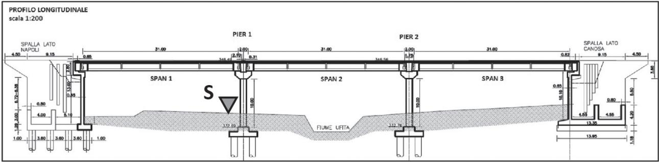
Fig. 2 – Longitudinal profile of the viaduct.
