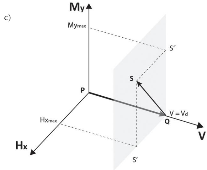
Fig. 11 – Load path in V- $H_x$ - $M_y$  space.
