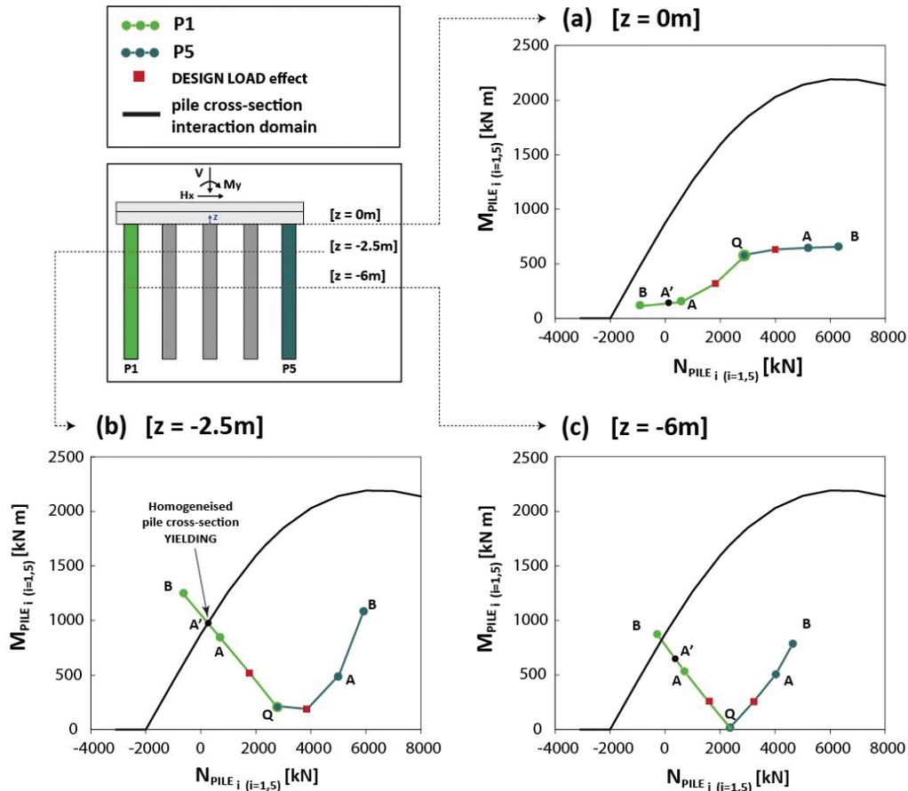
Fig. 17 – Generalized load paths for pile P1 and P5 at  $z=0m$ ,  $z=-2.5m$  and  $z=-6m$ .
