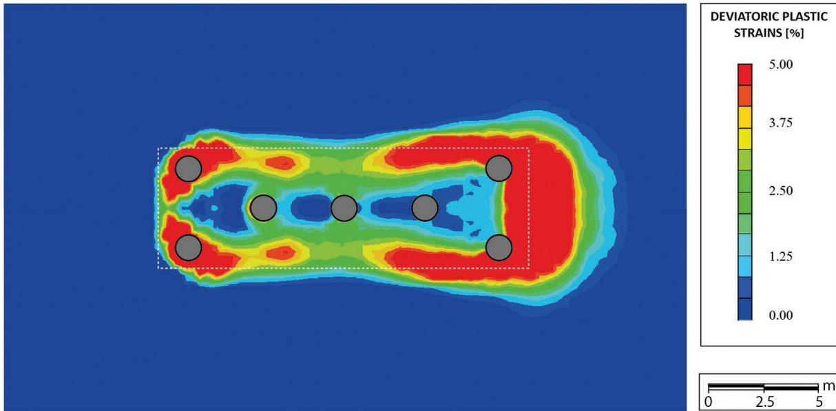
Fig. 14 – Plastic strain field in a cross-section at  $z=-2.5\text{m}$  at a load level correspondent to point F in Fig. 12.
