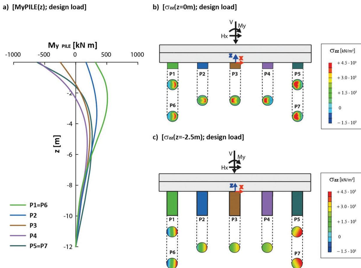
Fig. 16 – (a)  $M_{yPILE}$  along piles at design load (b) contours of vertical stresses in piles at pile head (c) contours of vertical stresses in piles at  $z=-2.5m$  (compression is assumed to be positive).
