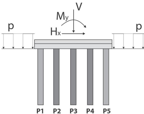
Fig. 6 – Geometrical scheme (longitudinal section) with applied loads.
