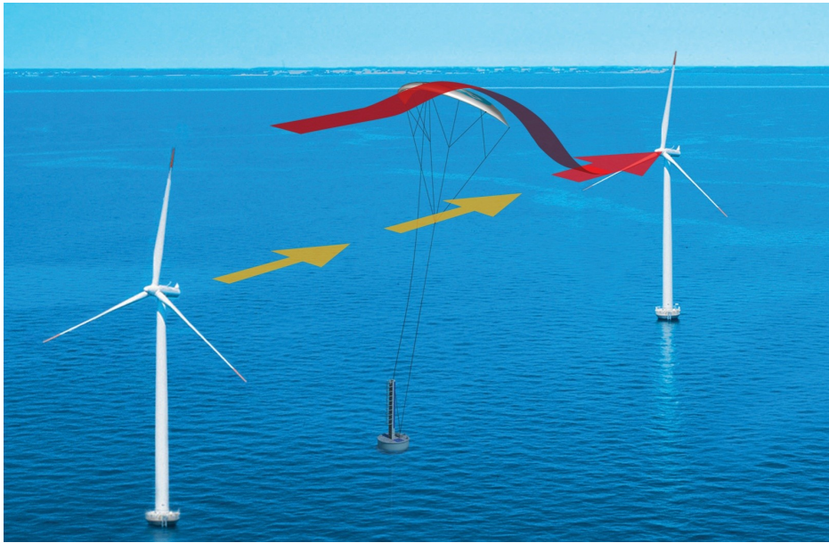
Figure 1.7: Proposed design for wind farm efficiency increase using a kite system to re-energy the wake (Boonman et al. [2011])
