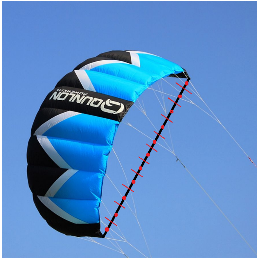
Figure 5.1: Representation of the actuator line method for a power kite. The kite is represented as a so called actuator line. Adapted from Bubba, O [2014] .
