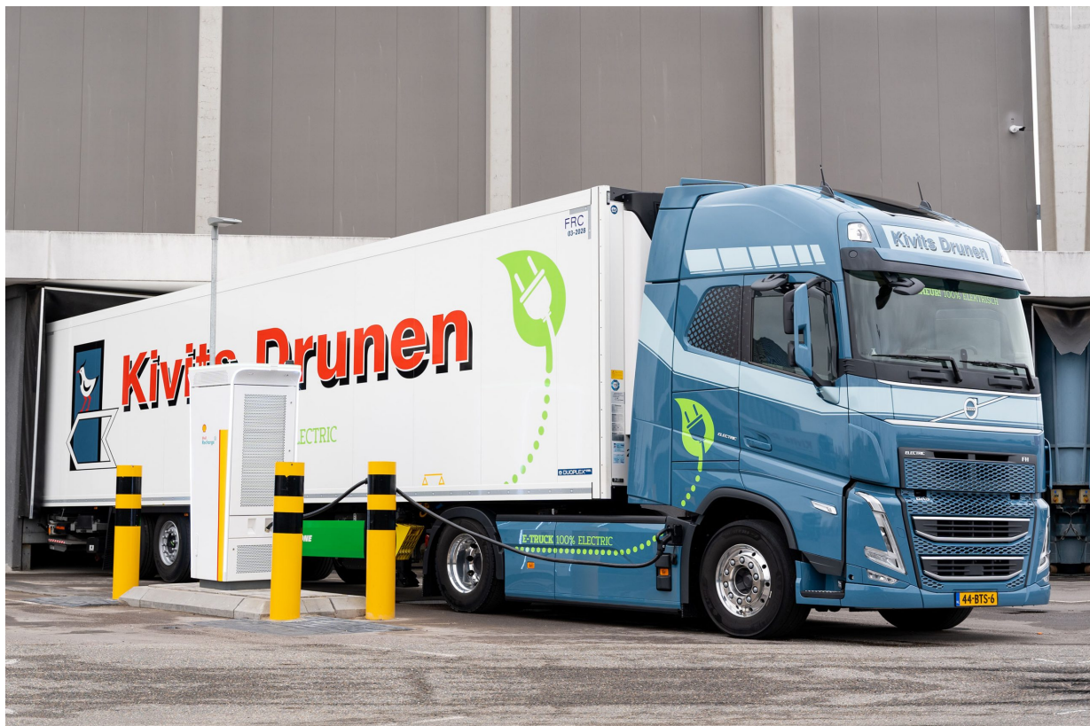
Figure 4.2: Volvo FH Electric Tractor coupled to a Shell AC Fast Charger. Image published by Shell
