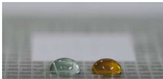
Figure: In-development, microfluidic robots developed at Volta Labs integrating electrowetting.
