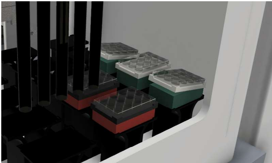
Figure102: Detail of the on deck warming plates and tilting plates.
