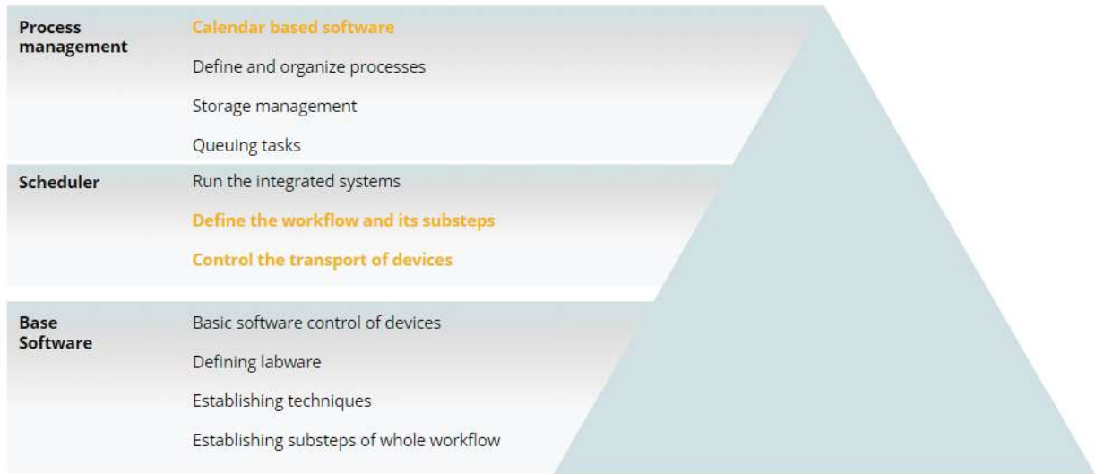
Figure 37: The structure of the software used by automating companies such as Beckman & Couter
