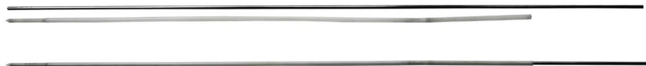
Figure 7 First steerable needle prototype (Top: stylet and sleeve separate, Bottom: stylet in sleeve)
