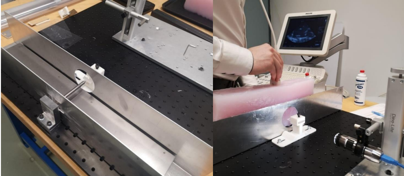
Figure 41 Final experimental setup (left: Steel calibration rod, right: phantom in shoot with ultrasound machine)
