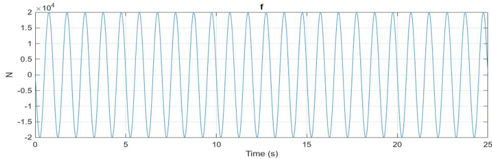
**Figure 4** Regular sine wave force input at the hydraulic cylinder 20kN
