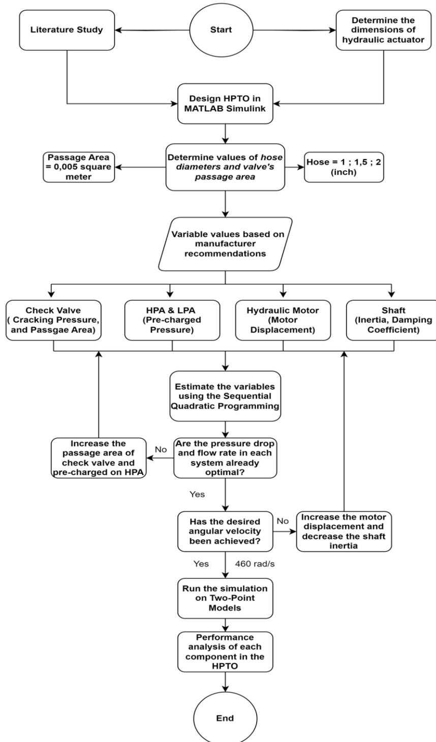
Figure 3 Flow chart of the HPTO optimization process
