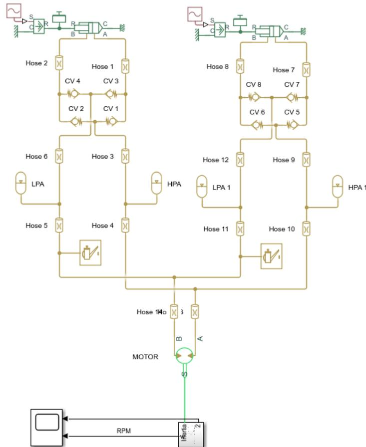
**Figure 7** Schematic of the Two-Point Absorber Model in Simulink presents a two-point absorber WEC system designed for enhanced energy capture. The model highlights the dual absorber configuration and its integration with the HPTO
