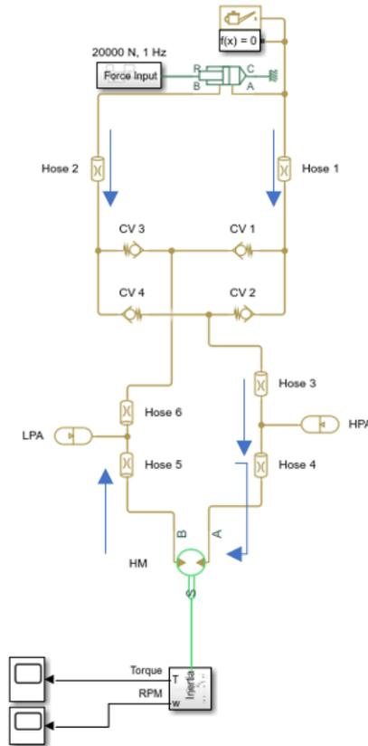
**Figure 6** Schematic of the Single-Point Absorber Model in Simulink illustrates the configuration of a single-point absorber Wave Energy Converter (WEC) integrated with a Hydraulic Power Take-Off (HPTO) system
