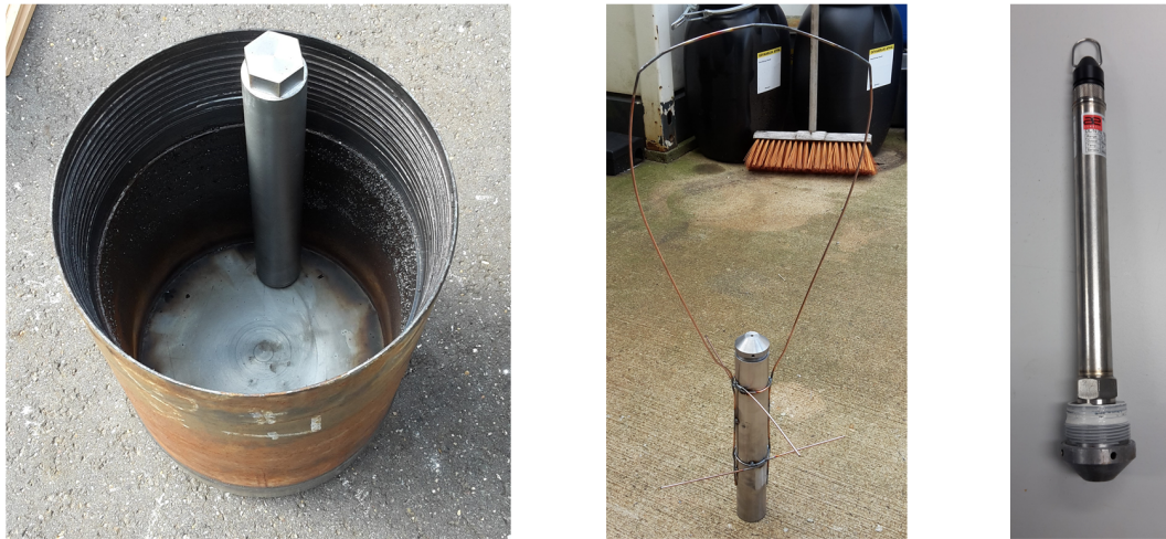
Figure E.6: Pressure sensor in the cone (left), pressure sensor for the bottom (middle), and a sensor without its protective housing (right)
