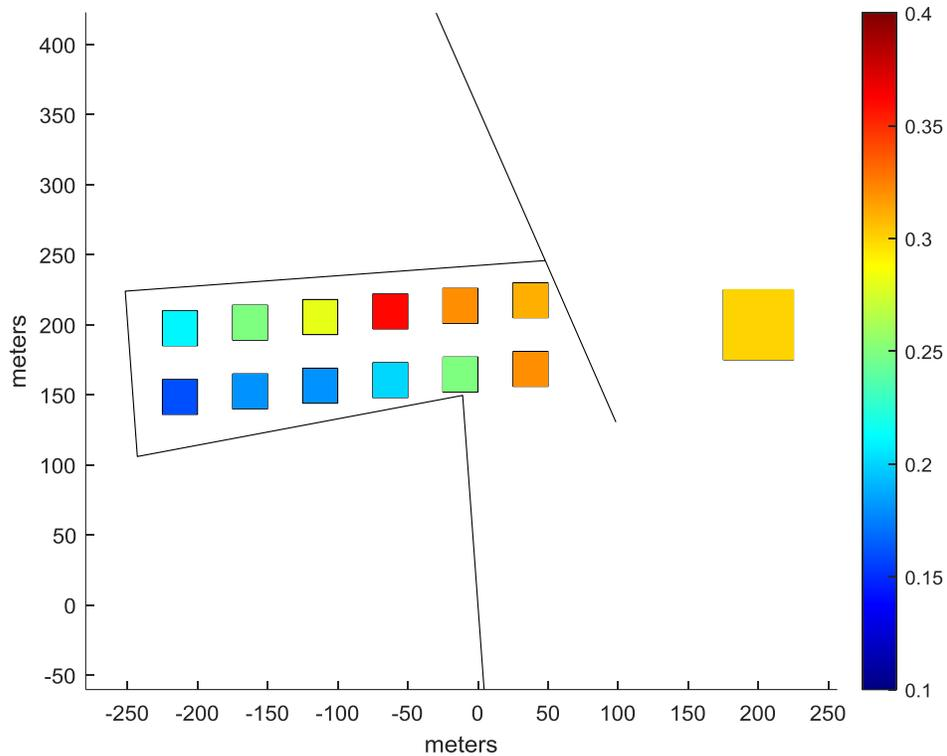
Figure 3.14: Wave height for the SLS conditions in SWAN
