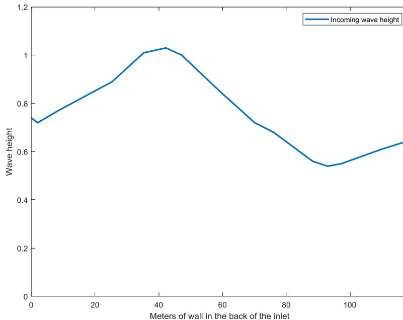
Figure 3.7: Incoming wave height projected on the wall at the back of the inlet for SLS conditions.
