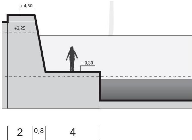
Figure 3.2: Provisional design vertical wall. The dotted line is NAP, with the values in the figure in meters related to NAP. The values underneath the figure are dimensions in meter.
