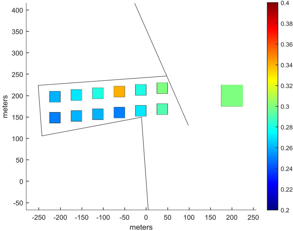
Figure 3.9: Wave height in the inlet for SLS conditions in SWASH.
