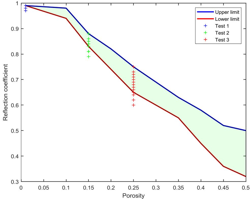
Figure 3.3: Results of the 1D SWASH computation with the different test results fitted in the reflection coefficient for a certain porosity. Parameters of the tests can be found in Table 2
