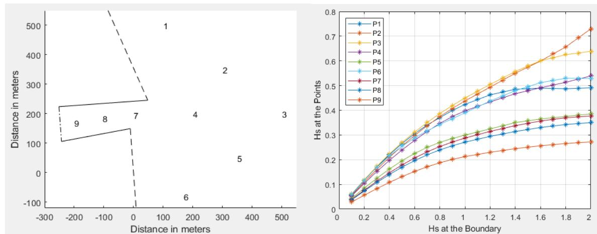
Figure 3.5: Left: locations of P1 to P9, dotted line for non-reflective wall, dot-stripe line for back wall which is in some cases non reflective. Right: relation Hs at the boundary and Hs at the locations P1 to P9.
