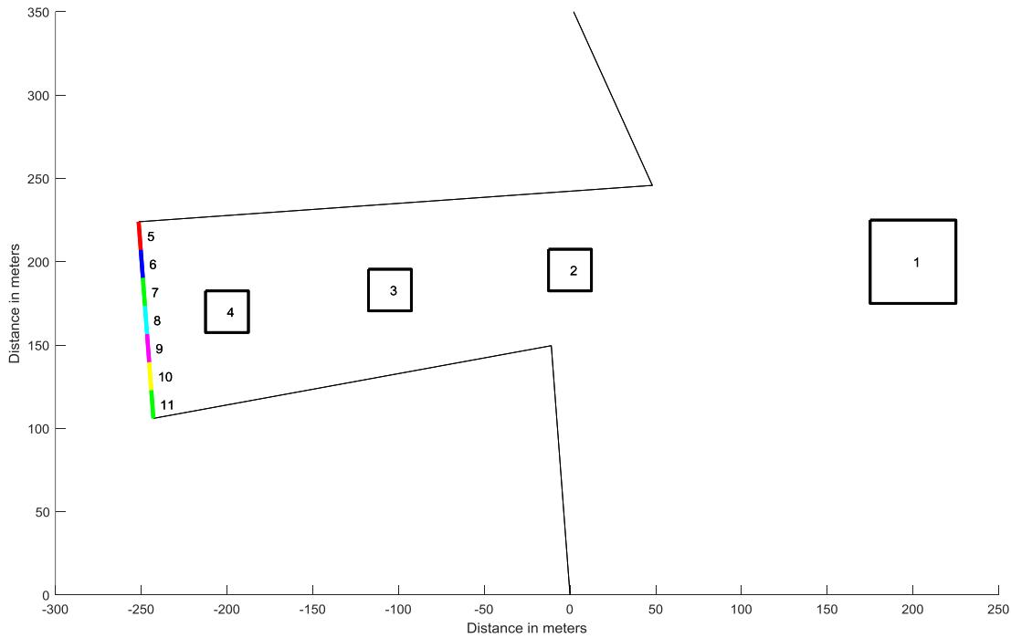
*Figure 3.6: Lay-out for the ULS simulation with areas 1 to 4 to determine the  $H_s$  outside and inside the inlet, and segment 5 to 11 to determine the wave height at the wall. North is pointed upwards.*
