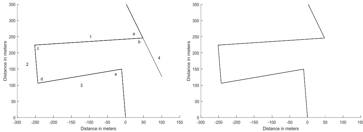
Figure 3.1 Inlet with breakwater (left) and without breakwater (right), with water on the right side of both figures and the north points upwards.
