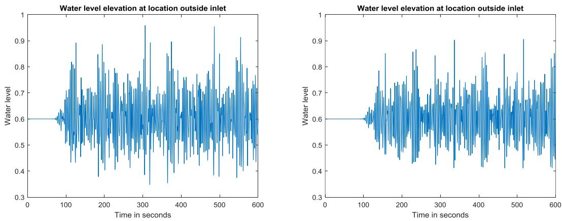
Figure 3.4: Water level elevation at location 200m outside the inlet (left) and just in front of the inlet (right)
