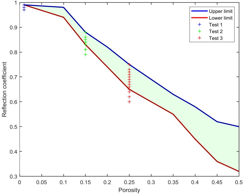
Figure 3.3: Results of the 1D SWASH computation with the different test results fitted in the reflection coefficient for a certain porosity. Parameters of the tests can be found in Table 2
