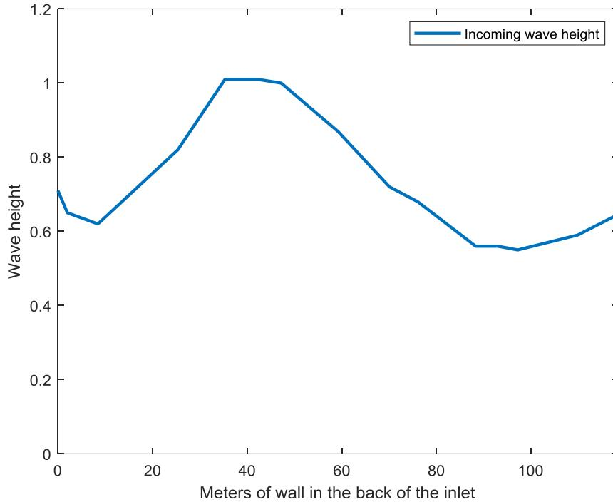
Figure 3.13: Incoming wave height projected on the wall at the back of the inlet for SLS conditions.
