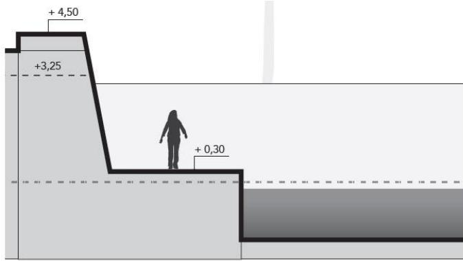
Figure 3.2: Provisional design vertical wall. The dotted line is NAP, with the values in the figure in meters related to NAP. The values underneath the figure are dimensions in meter.
