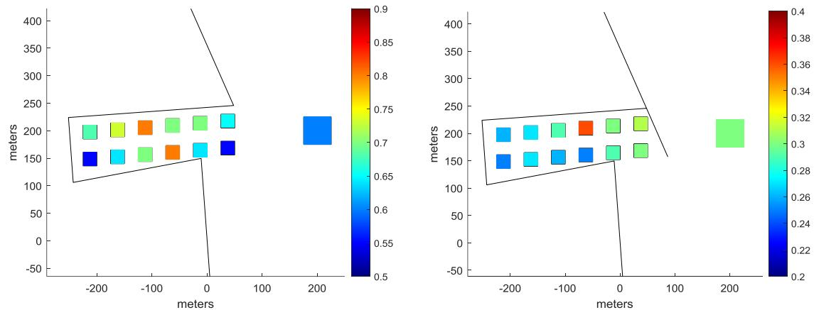
*Figure 3.12 : Wave height in the inlet during SLS conditions for the situation without breakwater (left) and with shorter breakwater (right).*
