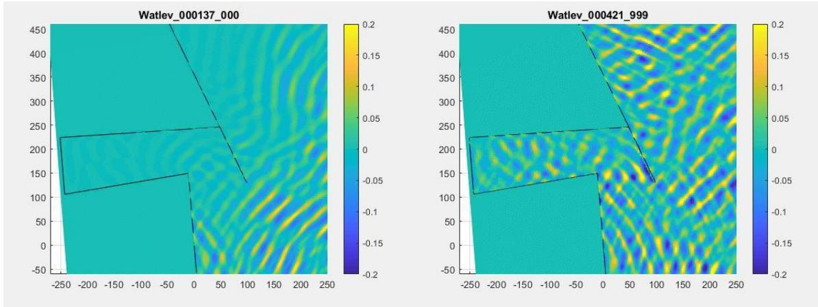
*Figure 5.2: Incoming waves mainly from one direction in the beginning of the simulation on the left, wave agitation in the inlet with waves going in all directions on the right.*
