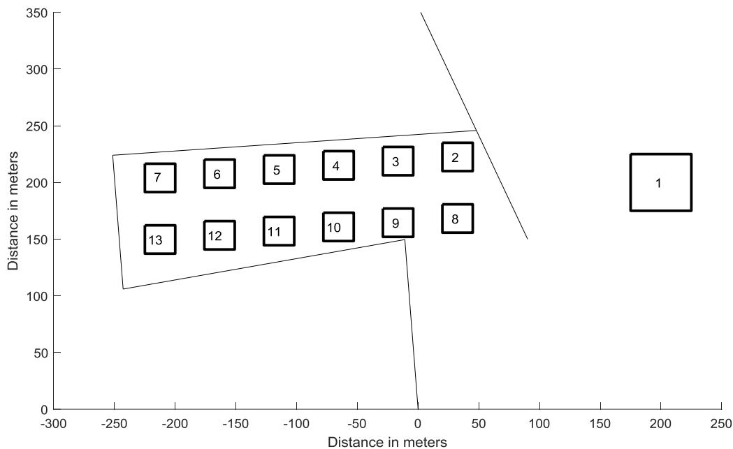
*Figure 3.11: Lay-out with 100m breakwater and locations 1 to 13 to determine the significant wave heights inside and outside the inlet.*
