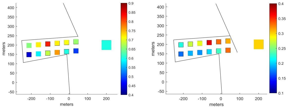
*Figure 3.15: Wave height in the inlet during SLS conditions for the situation without breakwater (left) and with shorter breakwater (right).*
