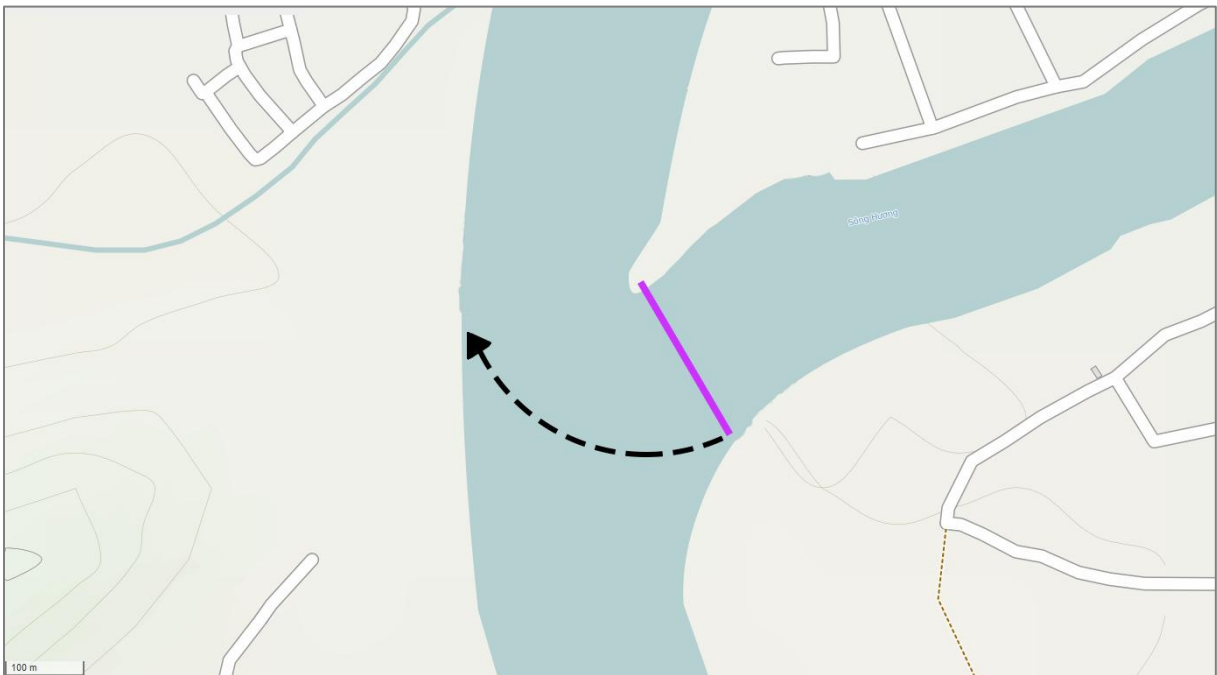
FIGURE 55: A TOP VIEW OF ROTATING GATE AT LOCATION 2
