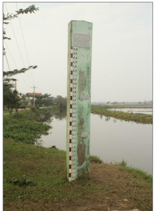
FIGURE 144: CONCRETE ROD TO READ THE WATER LEVEL IN TIMES OF FLOOD
