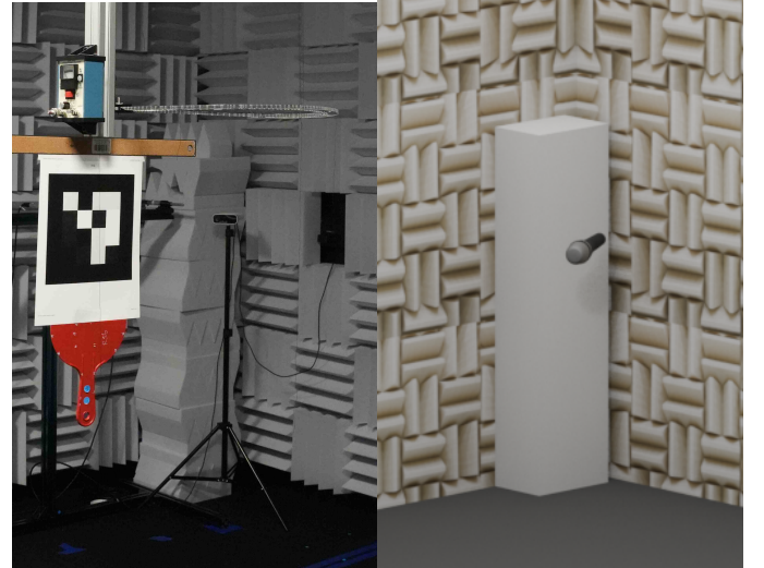
Fig. 17: Microphone 1 in the Treated Room (left) and in the simulated replica (right). In both rooms, a cuboid of absorptive material is placed on the right of the microphone, introducing room asymmetry. The left image is reprinted from [10].
