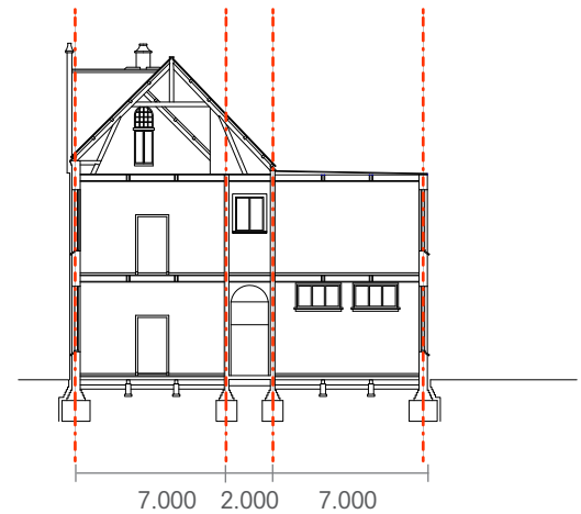
Figure 204 Structure - Section C-D, St. Anna
