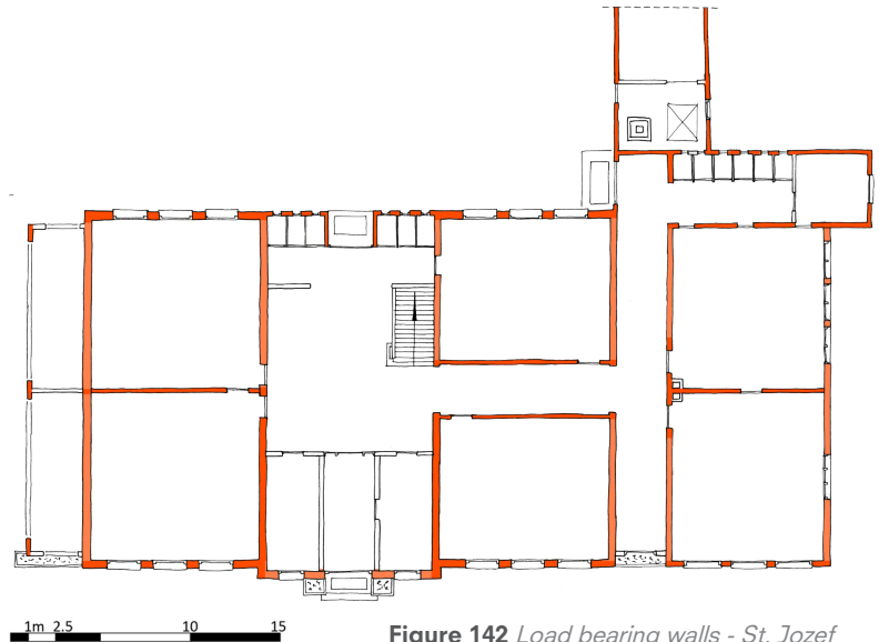
Figure 142 Load bearing walls - St. Jozef
