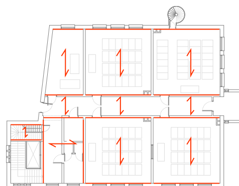
Figure 224 Floor Spans - First floor St. Anna
