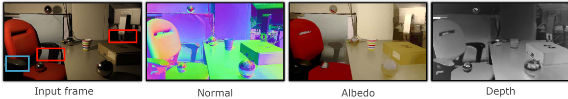
Fig. 21. Reconstruction results of the scene parameters for a complex, large scale real-world data set of an office work space. While a few artifacts occur in areas which are barely lit (red) or feature very dark materials (blue), most parts are truthfully reconstructed by our method.
