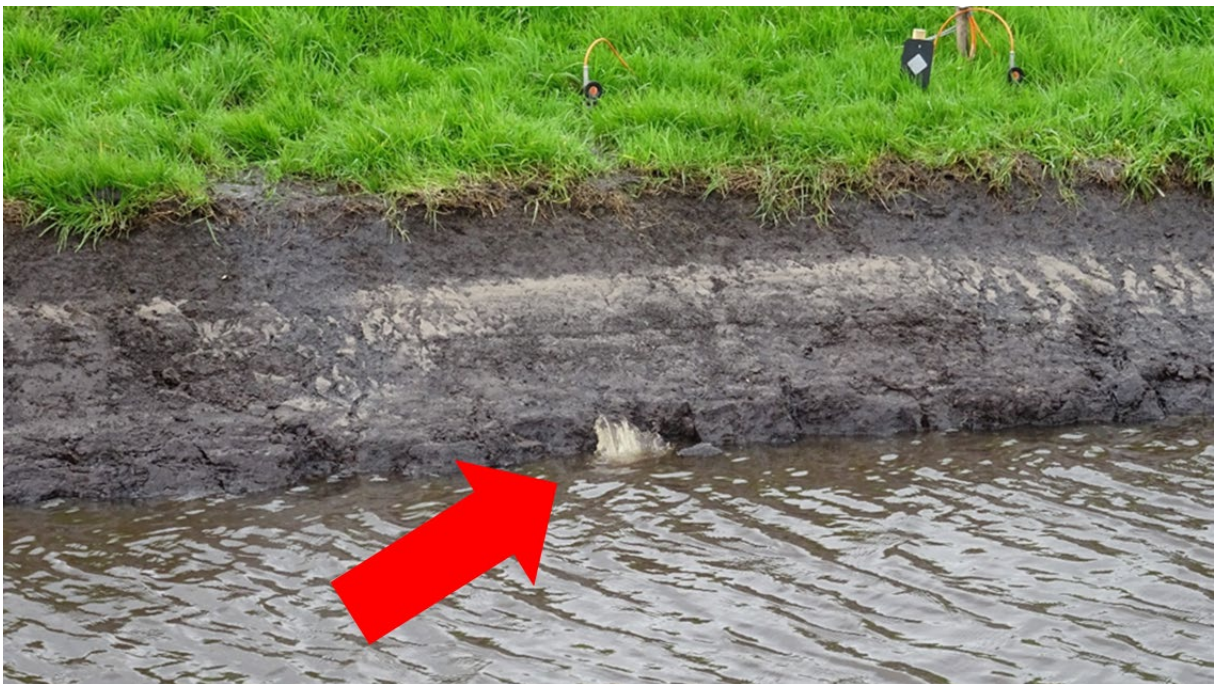
Figure 4.5 Significant amount of water draining from the peat layer as a result of the water level drawdown at the polder side of the levee running for a couple of hours.
