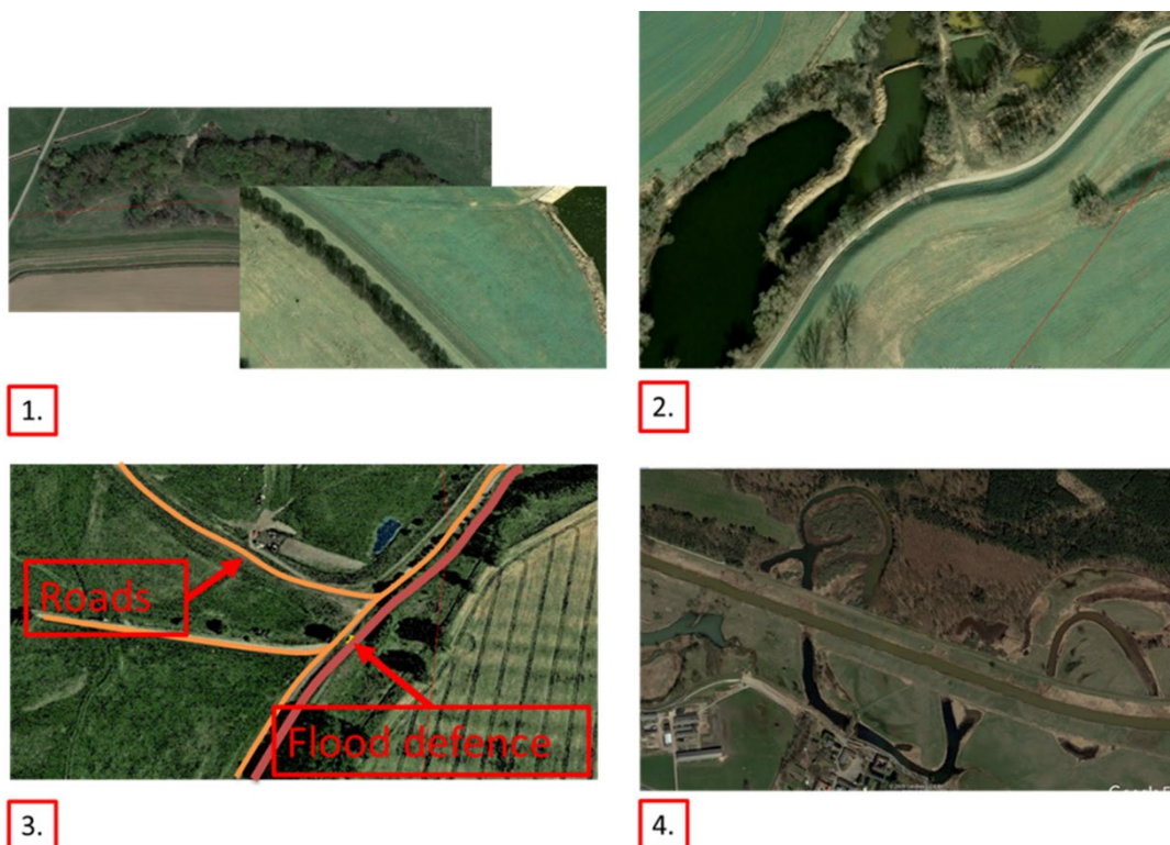
Figure 5.8 Illustration of deviating conditions (samples were taken from the Sachsen-Anhalt river system (Google, 2020a), 1: bushes or trees next to the levee, 2: permanent water directly next to the levee, 3: geometric changes of the cross-section of the levee (the road in orange on the levee in red branches off with several turns toward the river), 4: geological deviation observable in the subsurface, for example, old river belts
