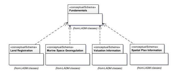
Figure 4 – Packages of the extended LADM with Marine Space, Valuation and Spatial Plan
