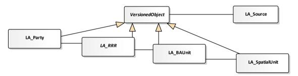
Figure 2 – Basic classes of the core LADM
