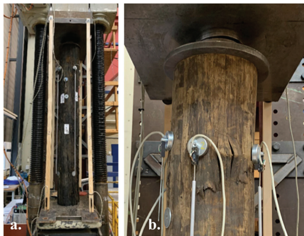
Fig. 9. a. Set-up for compression tests, b. LVDTs are mounted around knots.
