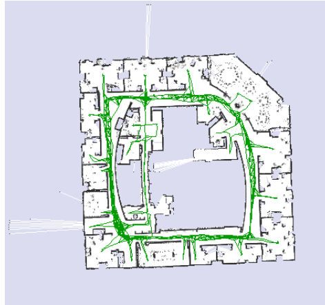
Figure 4-3: Occupancy grid derived from the data set of Intel Research Lab in Seattle [14].
