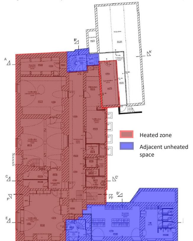
Figure 41: Floor plan cellar, heated zones (Source: NIBE, 2008)
