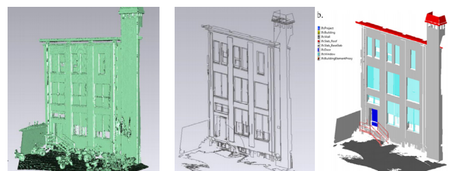
Figure 14: From pointcloud into BIM model (Source: Previtali)
