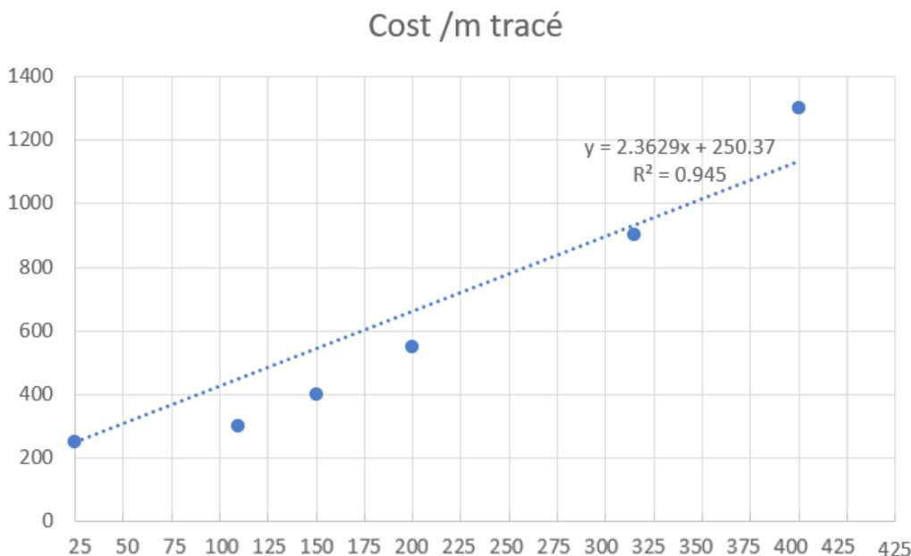
Figure A.1 - Cost estimation graph cost per pipe length
