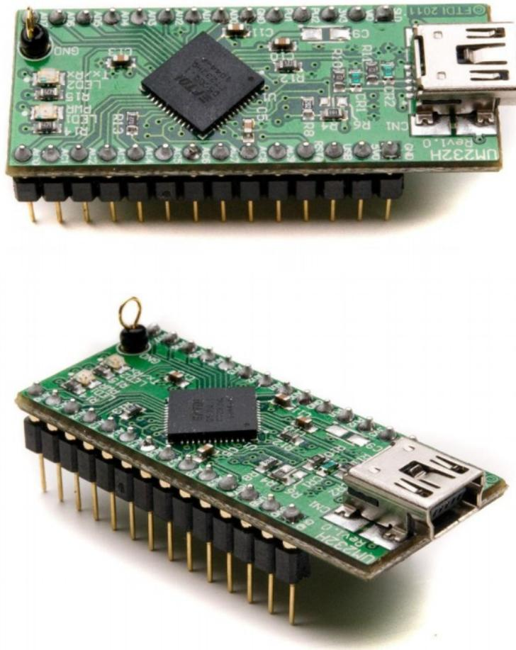
Figure C.1: UM232H USB to Serial/FIFO Development Module [36].
