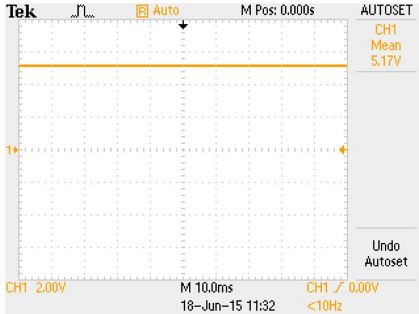
Figure C.15: Mean value of  $V_{\text{REGIN}}$ .
