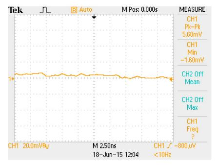
Figure C.12: Ripple of V<sub>REF</sub>.
