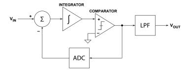
Figure 3.3: Block diagram of a Delta-Sigma modulator on a high level [25].
