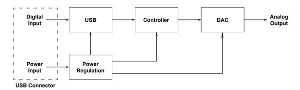
Figure 3.1: Block diagram of the USB DAC.
