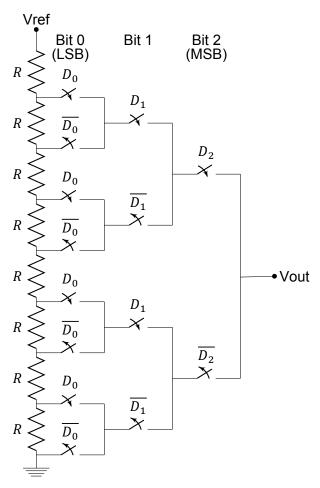
Figure 3.7: Architecture of a 3-bit R-string DAC.
