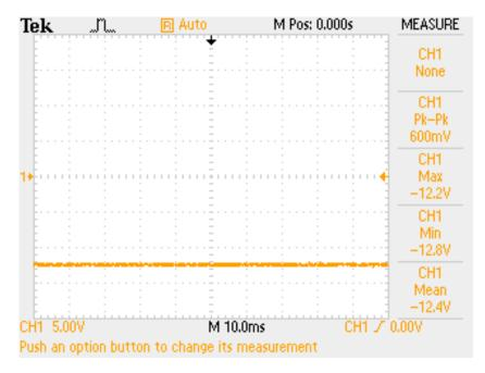
Figure C.17: Mean value of  $V_{SS}$ .
