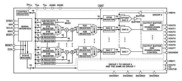
Figure 4.6: AD5370 block diagram [40].
