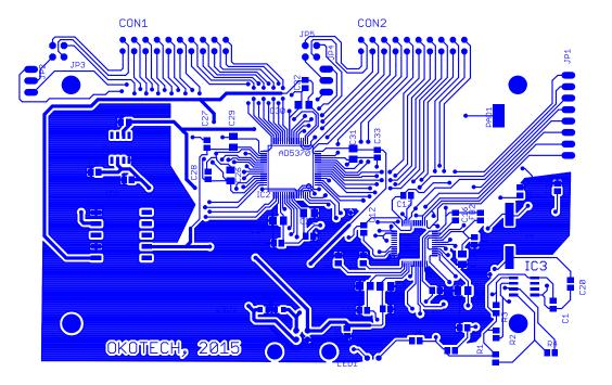
Figure C.5: The top copper layer of the PCB, visualized using the Gerber files.
