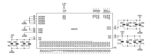
Figure 4.11: Schematic of the DAC connection diagram.
