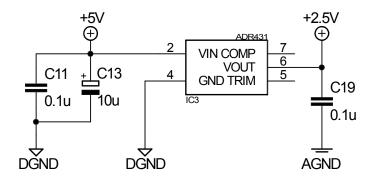
Figure 4.14: Schematic of the ADR431B.
