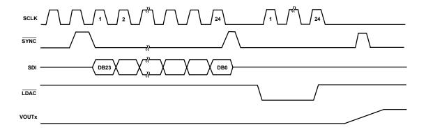
Figure 4.8: SPI write timing diagram of the AD5370 [40].
