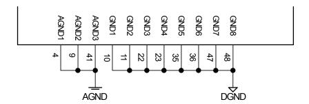
Figure 4.2: First part of the schematic of the FT232H showing the grounding.
