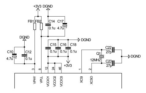
Figure 4.5: Fourth part of the schematic of the FT232H.
