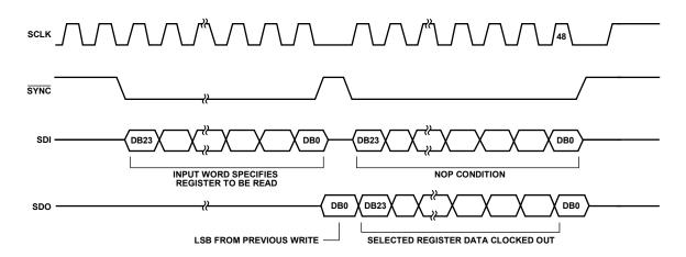
Figure 4.9: SPI read timing diagram of the AD5370 [40].
