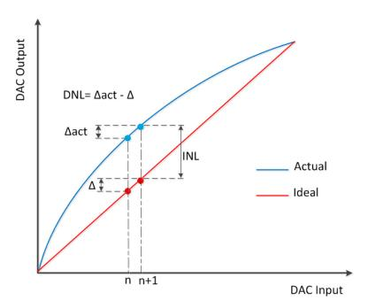
Figure 4.10: Figure illustrating the integral nonlinearity and differential nonlinearity [41].
