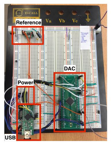
Figure 4.17: The prototype on a breadboard.
