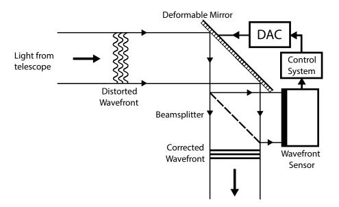
Figure 2.1: Basic adaptive optics measurement setup [4].
