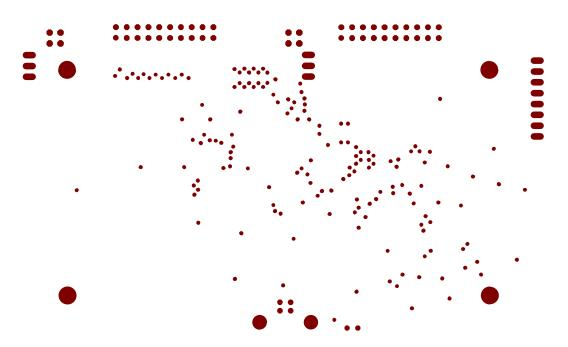
Figure C.7: The exposed parts of the bottom layer of the PCB, visualized using the Gerber files.
