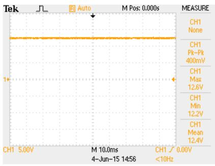
Figure C.18: Mean value of  $V_{\text{DD}}$ .
