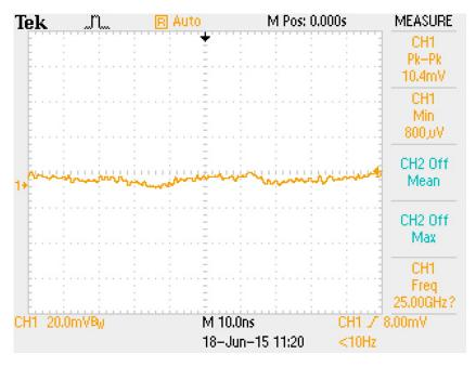
Figure C.14: Ripple of DV<sub>CC</sub>.
