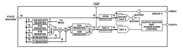
Figure 4.7: Block diagram of a single DAC channel of the AD5370 [40].
