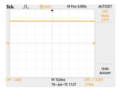
Figure C.11: Mean value of  $V_{\text{REF}}$ .
