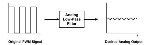
Figure 3.4: Block Diagram of a PWM DAC conversion [28].
