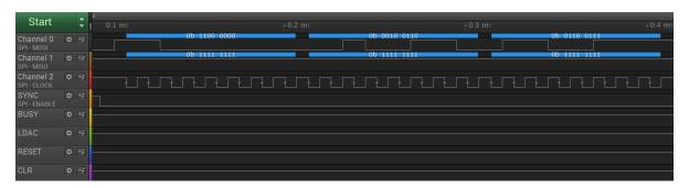
Figure 4.16: Example of SPI signals on logic analyzer.
