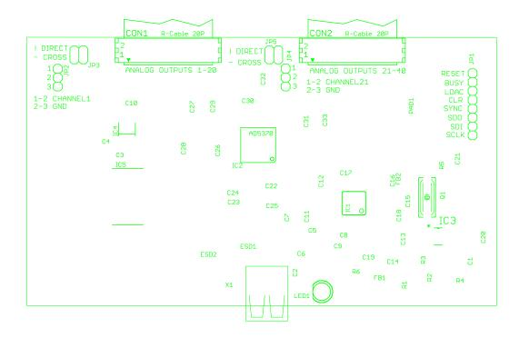
Figure C.4: The text layer of the PCB, visualized using the Gerber files.
