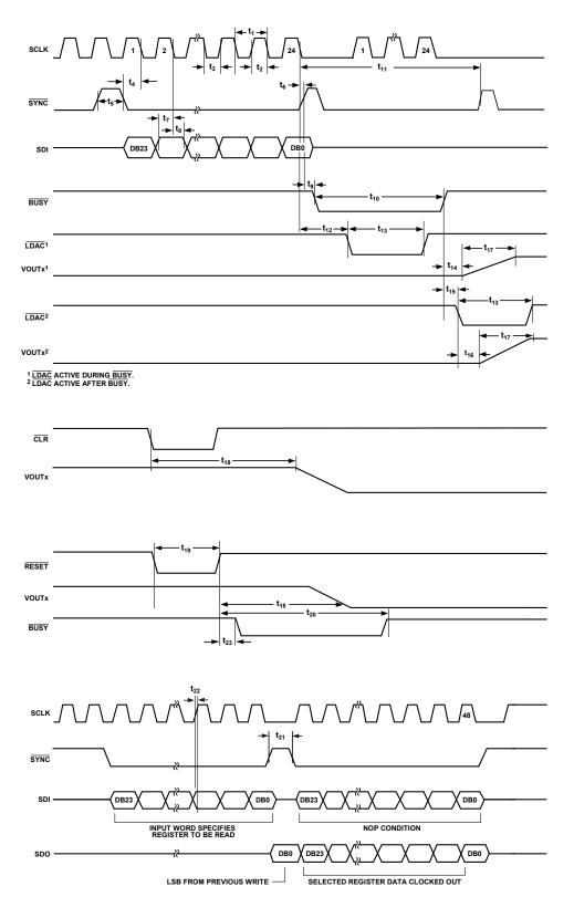
Figure C.2: AD5370 SPI interface write and read timing diagram [40].
