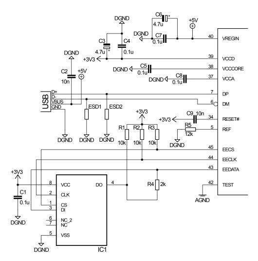
Figure 4.4: Third part of the schematic of the FT232H.
