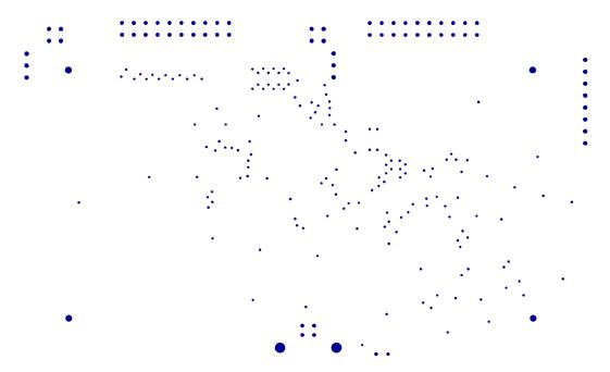
Figure C.8: The drill hole layer of the PCB, visualized using the Gerber files.
