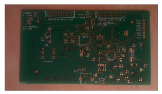
Figure C.10: PCB design, manufactured by Eurocircuits, without components soldered on it.
