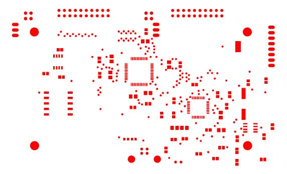
Figure C.6: The exposed parts of the top layer of the PCB, visualized using the Gerber files.
