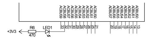
Figure 4.3: Second part of the schematic of the FT232H showing the output pins.
