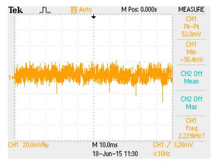
Figure C.16: Ripple of V<sub>REGIN</sub>.
