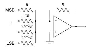
Figure 3.5: Architecture of a N-bit binary weighted DAC.
