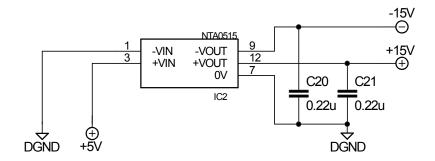
Figure 4.15: Schematic of the NTA0515MC.
