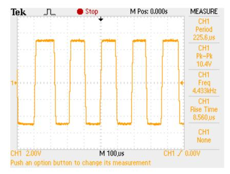
Figure 5.1: Analog output refresh rate measurement.
