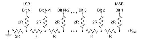
Figure 3.6: Architecture of a R2R DAC with N bits [32].
