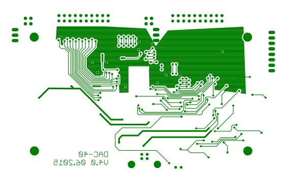
Figure C.9: The bottom copper layer of the PCB, visualized using the Gerber files.
