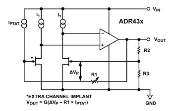
Figure 4.12: Schematic of the precision converter [43].
