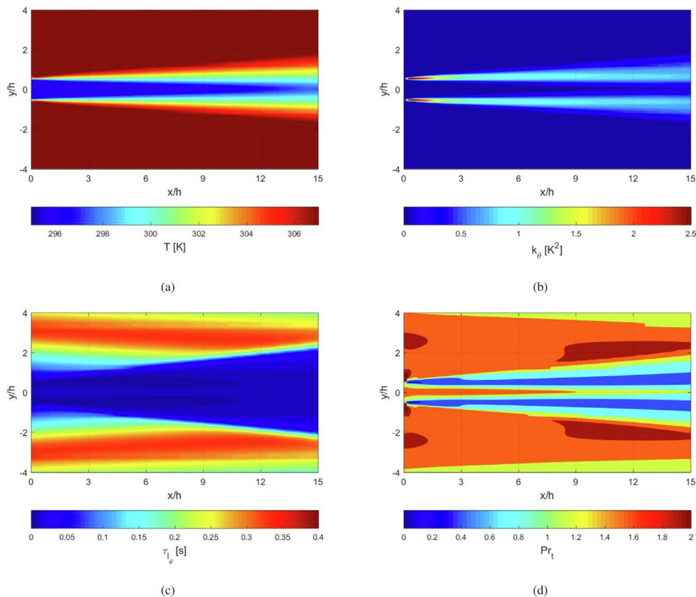
**Fig. 5.** Contours of temperature (a), temperature variance (b), local thermal time scale (c) and turbulent Prandtl number (d) at  $Pr = 0.2$ , obtained from the low-Reynolds  $(k - \varepsilon - \zeta - f) + (k_\theta - \varepsilon_\theta)$  turbulence model (domain D2.1).
