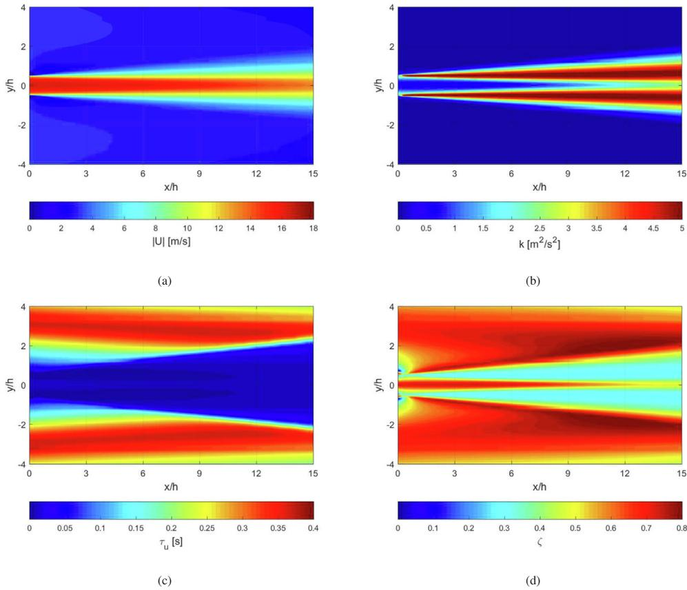
**Fig. 4.** Contours of velocity magnitude (a), turbulent kinetic energy (b), global dynamical time-scale (c) and velocity-scale ratio (d) from the low-Reynolds  $(k - \varepsilon - \zeta - f) + (k_\theta - \varepsilon_\theta)$  turbulence model (domain D2.1).
