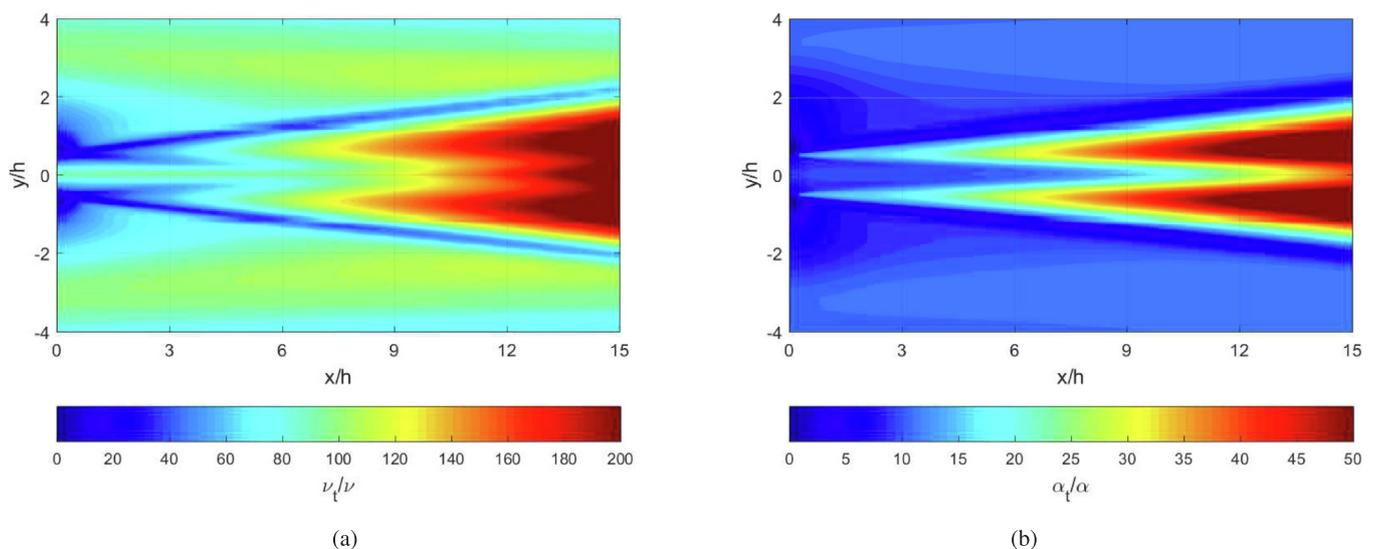
**Fig. 6.** Contours of turbulent to molecular viscosity (a) and diffusivity (b) ratios at  $Pr = 0.2$ , obtained from the low-Reynolds  $(k - \varepsilon - \zeta - f) + (k_\theta - \varepsilon_\theta)$  turbulence model (domain D2.1).
