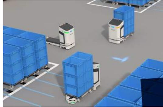
(b) Multiple Active Shuttle AGVs navigating an intersection while carrying payloads (blue crates).
