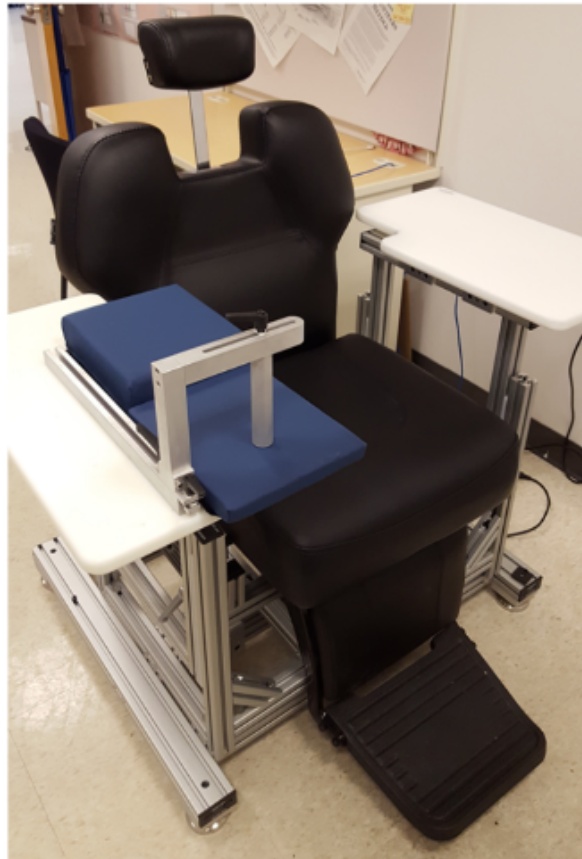
Figure 2.6: The chair and side tables used for the H-reflex screening. This setup is especially designed according to the needs of the H-reflex operant conditioning protocol. In other words, the height and the proximity of the side tables to the chair as well as, the hand peg are adjustable, so that the same setup can be used by multiple individuals.
