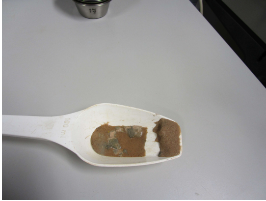
(a) Crushed material (grey) as found in the course of the CPT rod
