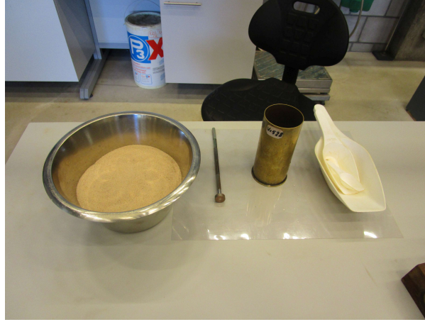
Figure G.7: Equipment needed for determination of the minimum and maximum sand density, the balance has not been included in the photo
