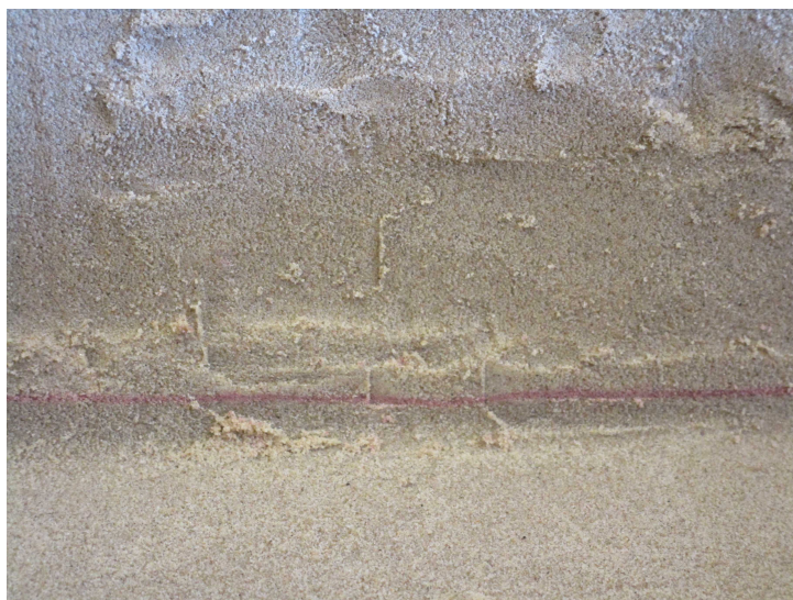
Figure G.52: Photo of excavation of the layer with coloured sand
