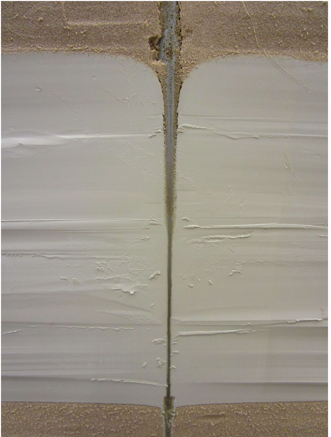
Figure I.2: Detail of the clay layer of the cross-section of sample 2
