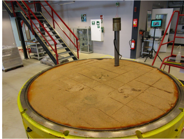
Figure G.32: Bulge on the surface caused by expansion of the sample due to penetration
