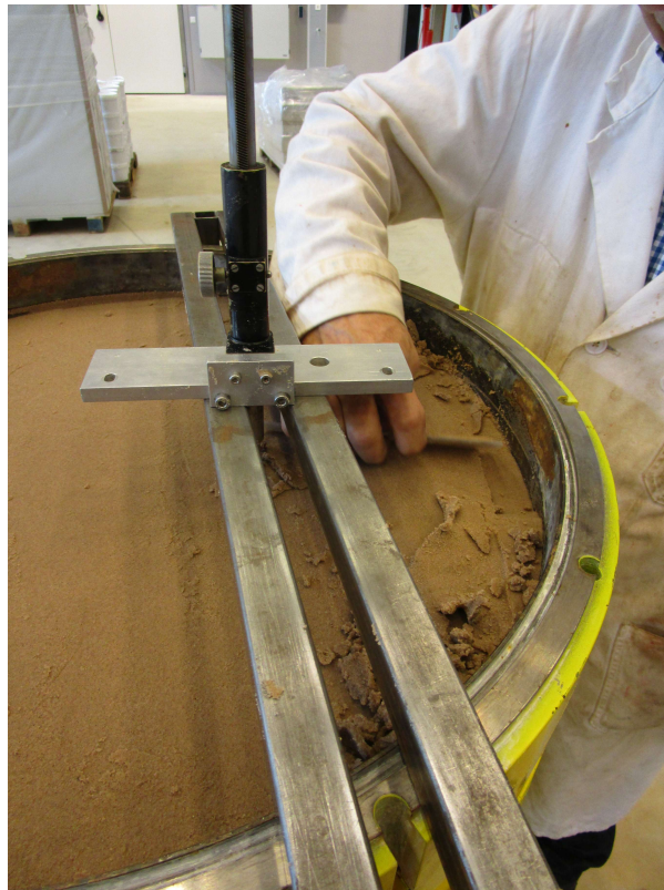
Figure G.16: Sand trimming technique for achieving a flat surface
