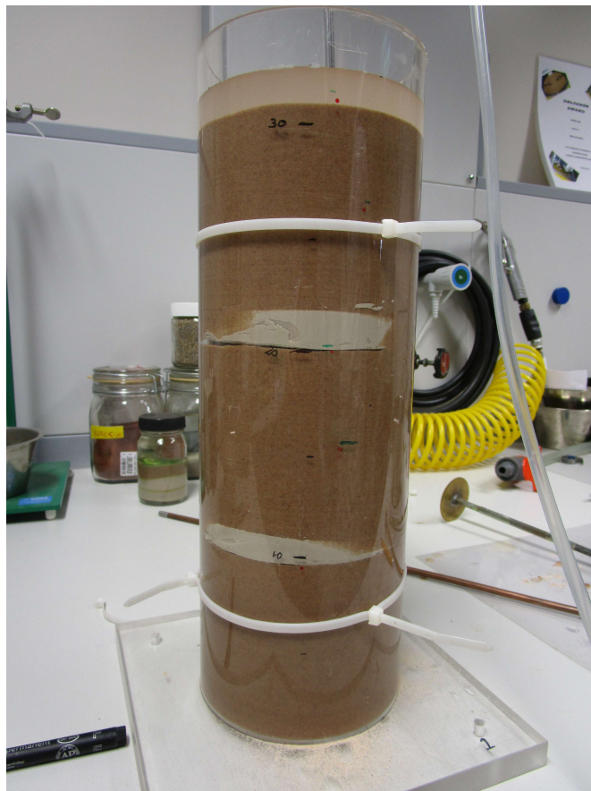
Figure G.14: Experimental setup for investigating preparation method for building a layered sample
