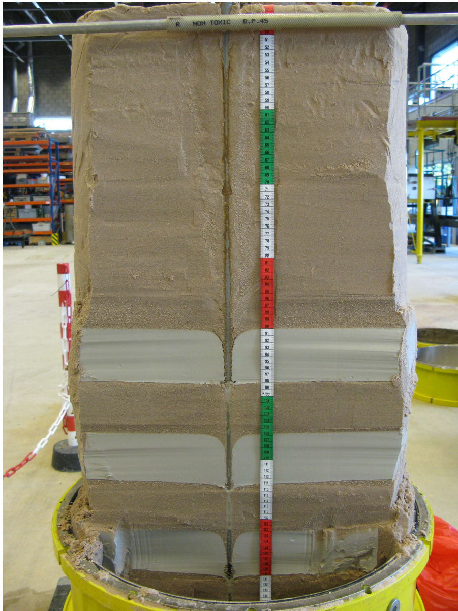
Figure G.58: Overview of the cross-section during sample dismantling
