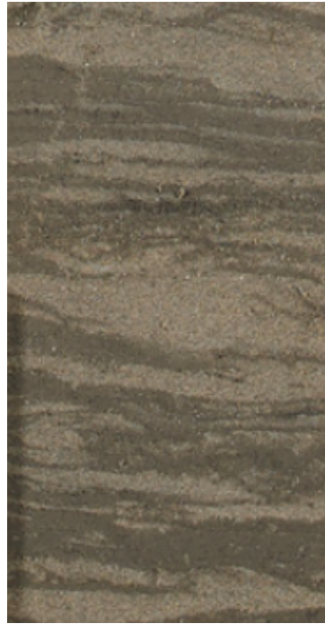
Figure 1.2: Detail from a borehole log containing flaser bedding deposits
