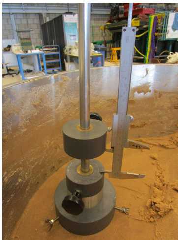
(a) Sampling cylinder with scraper
