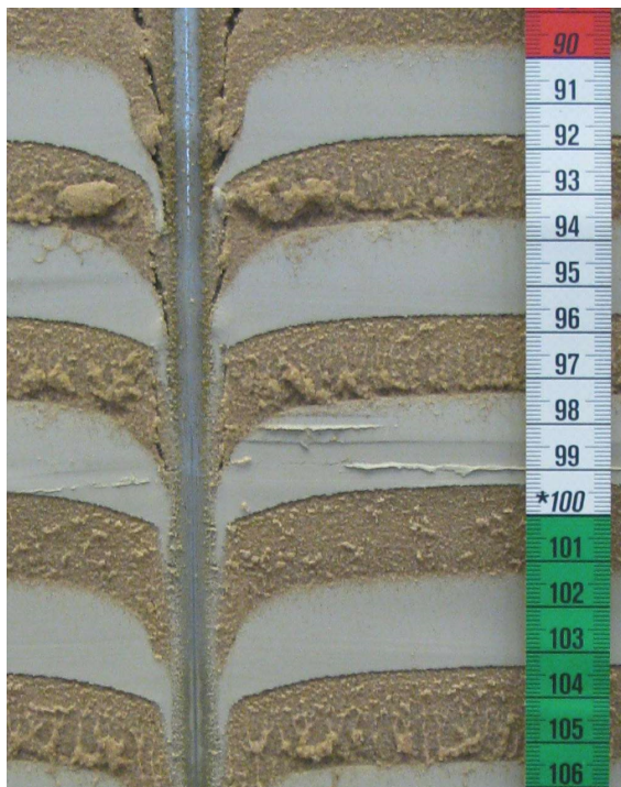
(a) Detail along the cone rod with horizontal thin clay lenses highlighted in red
