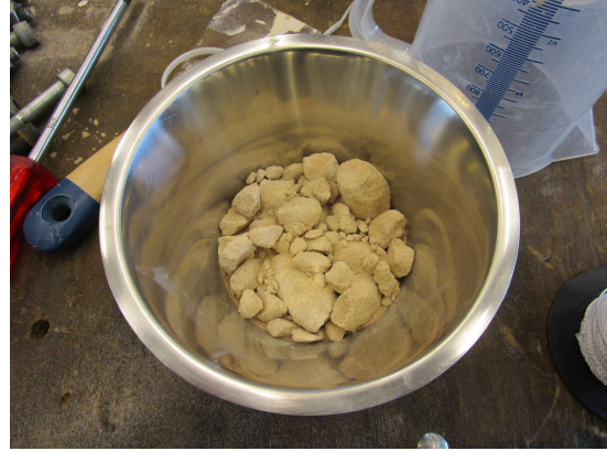
(b) Crushed material as obtained after drying of the sand
