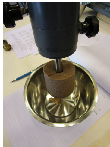
(b) Density sample taken out of the sampler
