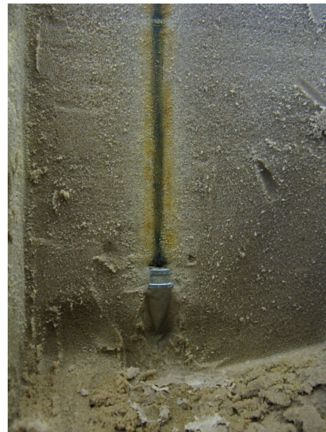
(b) Cross section of sample 1 near the cone tip
