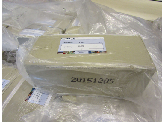
Figure G.17: Original clay brick sealed with the batch serial number printed on the side of the packaging
