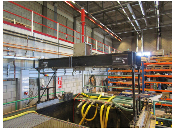
(b) Driving plunger, frame and tank in which the cell containing the sample was placed
