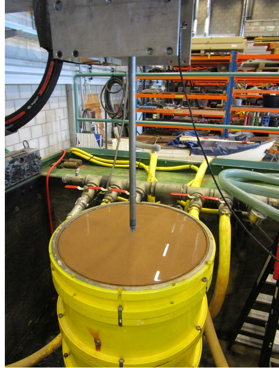
(a) Equipment configuration for tests on the first sample (b) A sample about to be penetrated for penetration testing
