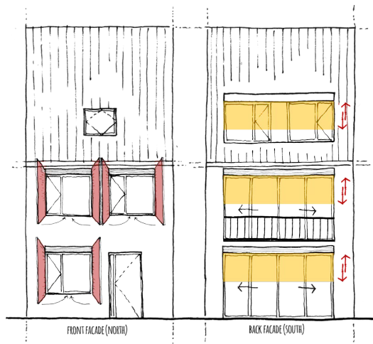
FIGURE 7.5 Optimisation of the façade increasing the glass percentage of the South using screens or awnings for adaptive solar gain on the South façade and thermal hatches on the North façade.
