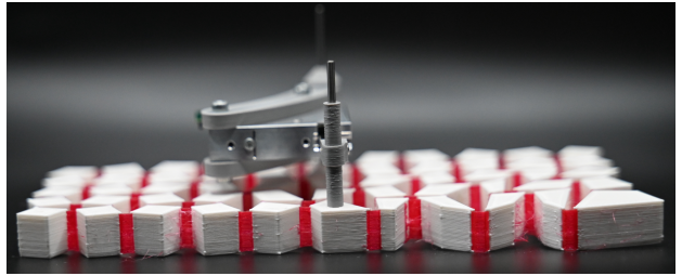
(d) Single metamaterial 3D print, with press-fitted steel pin ( \phi 2 \times 50 \text{ mm} ) into the lower actuated block, one spacer, the actuator slid over the pin, and the second spacer.
