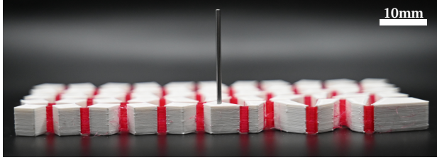
(a) Single metamaterial 3D print, with press-fitted steel pin ( \phi 2 \times 50 \text{ mm} ) into the lower actuated block
