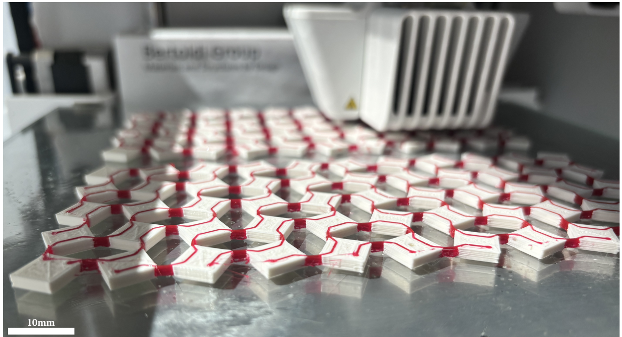
Fig. 14. Perspective view on the PLA and TPU 3D printing process.
