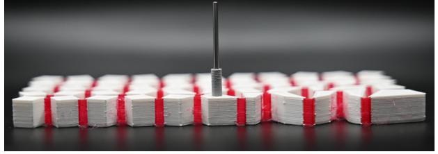
(b) Single metamaterial 3D print, with press-fitted steel pin ( \phi 2 \times 50 \text{ mm} ) into the lower actuated block, and one spacer
