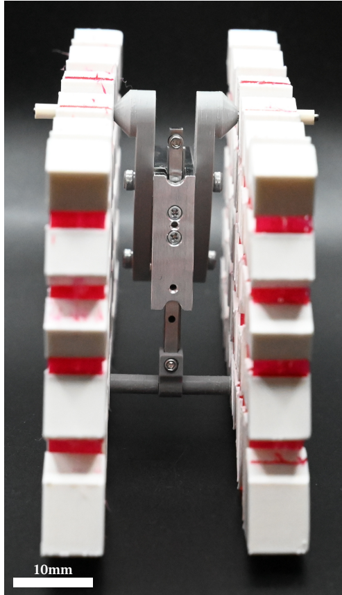
(a) Front view of the robotic prototype, showing the actuator sandwiched between the metamaterials.
