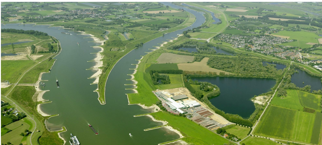
Figure 1.1: Aerial photograph of groynes in the river Waal and the Pannerdensch canal, (source: Rijkswaterstaat).
