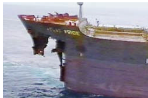
Fig 1-2 Bow damage on the supertanker "Atlas Pride" due to a freak wave
