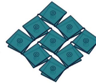
materialization hinge thickness: 0.7 mm rigid panels thickness: 3 mm height: 13 mm
