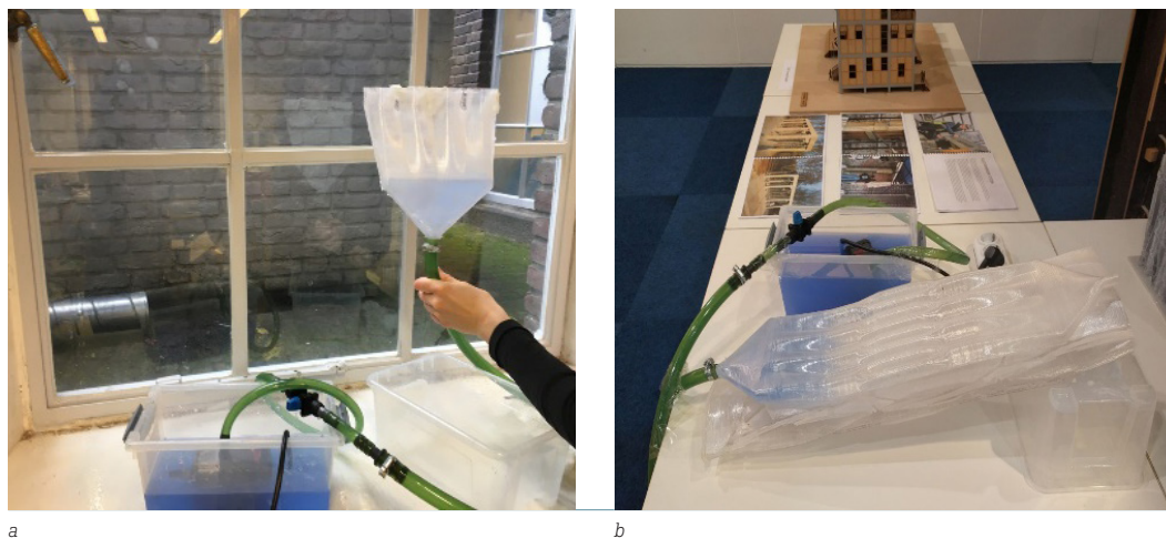
FIG. 5 Water circulation test in the external layer
