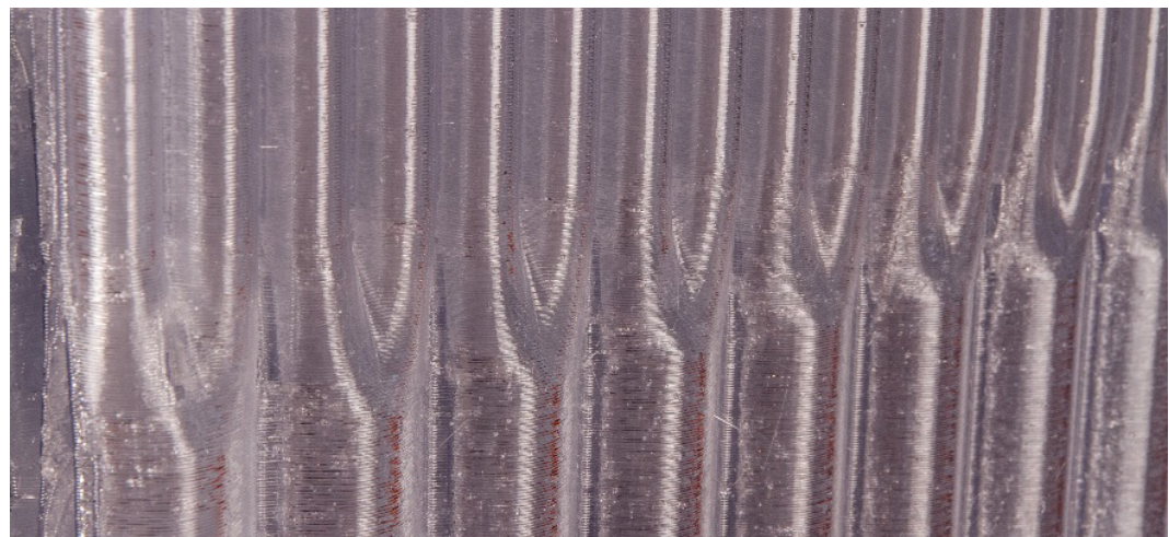
FIG. 4 Printed segment of the external layer
