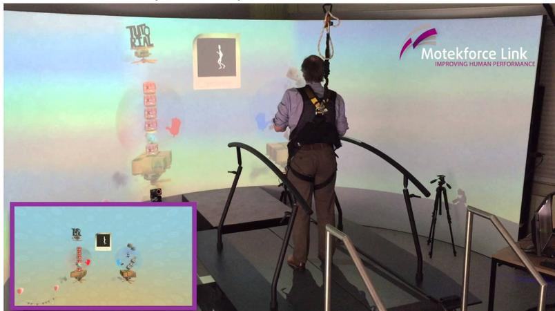
Figure 1. Treadmill, virtual reality environment and safety harness
