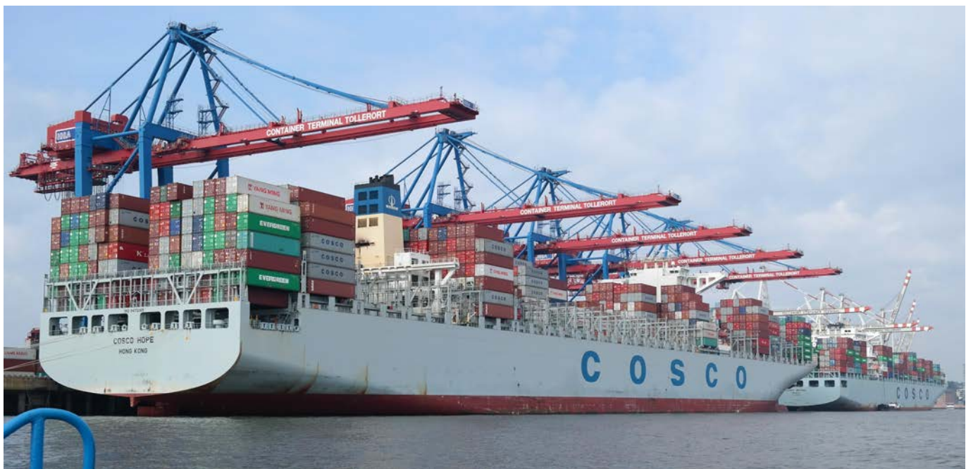
Figure 4.17: 21,000 TEU COSCO Development being handled by six STS cranes at Euromax terminal in the port of Rotterdam (SIF W & COSCO NEBULA by kees torn is licenced under CC BY-SA 2.0).
