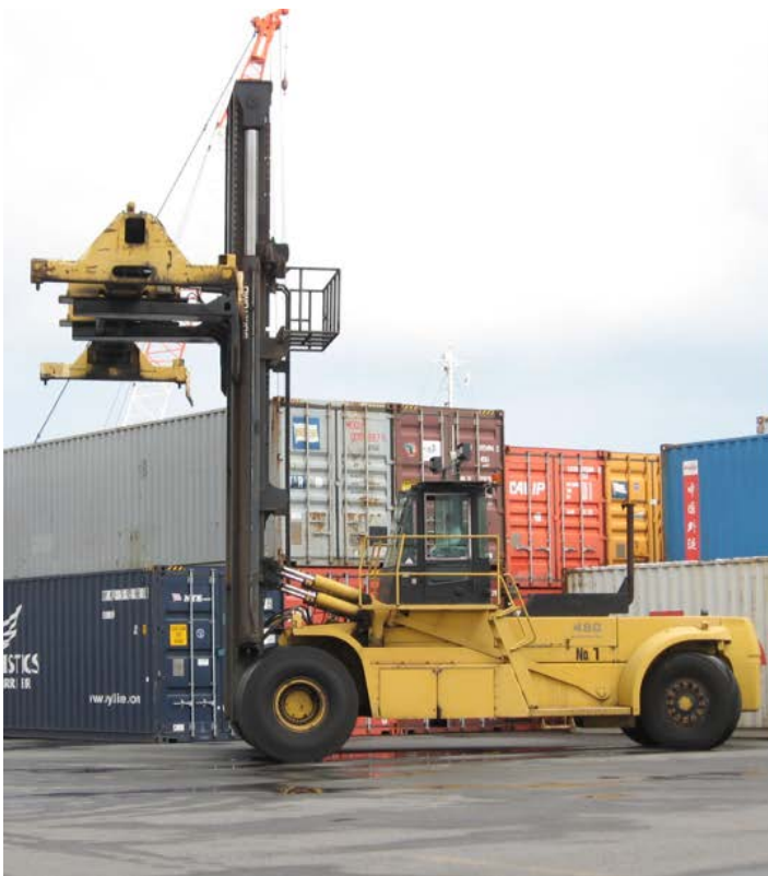
Figure 4.18: Container handling equipment; left: toploader (by Gazouya-japan is licenced under CC BY-SA 4.0); right: reach stacker (by NAC is licenced under CC BY-SA 4.0).
