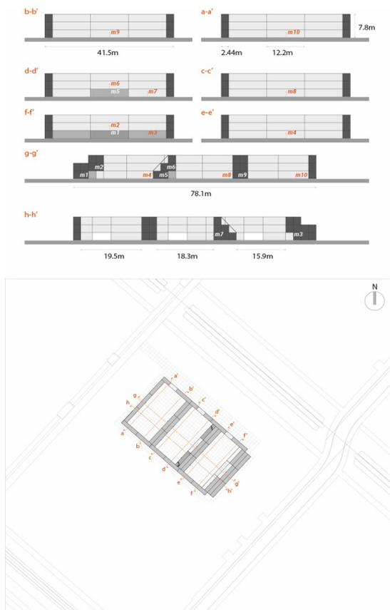
Figure 4 (top): Cross-section of the Urban Comfort Lab showing the size of the courtyards and location of microphones. Microphones 5-8 are in the experimental courtyard, while microphone 11 is on the roof. Taken from Lugten 2023.
