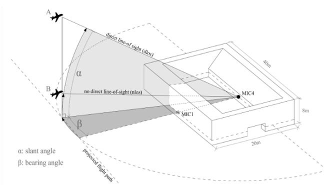
Figure 6: Diagram showing slant angle and bearing angle of aircraft relative to a simulated courtyard of the Urban Comfort Lab. Taken from Wuite et al. 2023.
