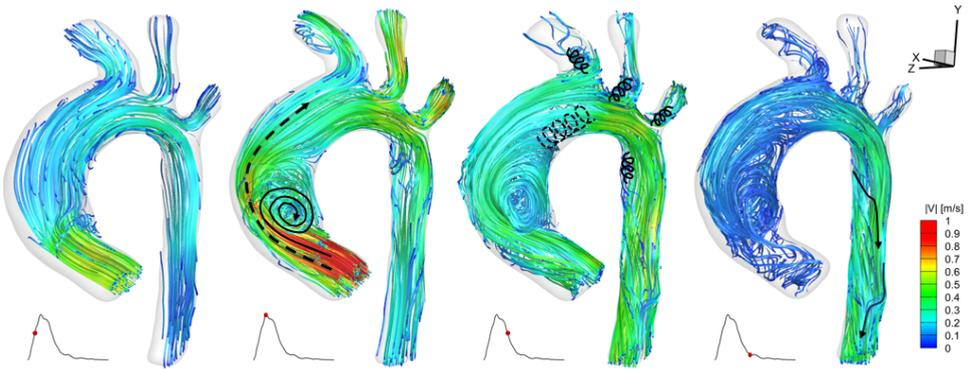
Figure 4.5: 3D streamlines of the aorta phantom at four key-frames of the cardiac cycle (mid acceleration, peak systole, mid deceleration, and early diastole), colored by velocity magnitude.
