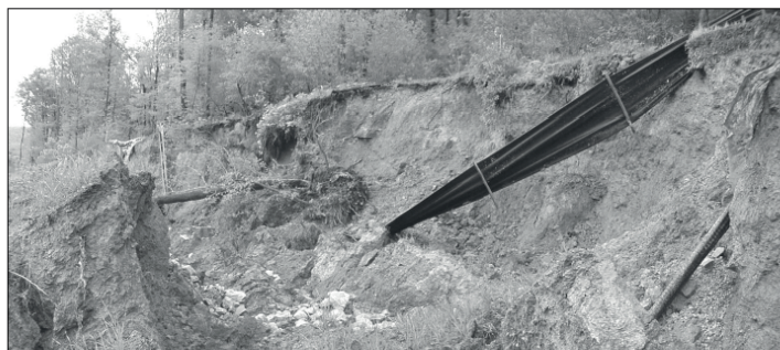
(b) View of 7.6 meter tall main scarp.
