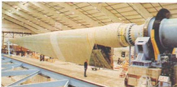
Figure 2.26: Filament winding set-up for blade manufacturing at Hamilton Standard [22].
