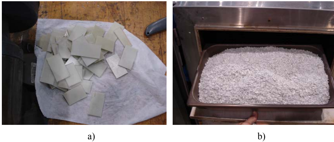
Figure 4.13: Raw material shredding. a) Trimmed and cut laminate to be fed to the granulator. b) Recyclate being oven dried prior to injection.
