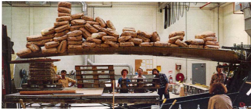
Figure 2.43: Økær 7.5m blade under static testing at Risø laboratories to validate the steel flange root design, 1982 [36].
