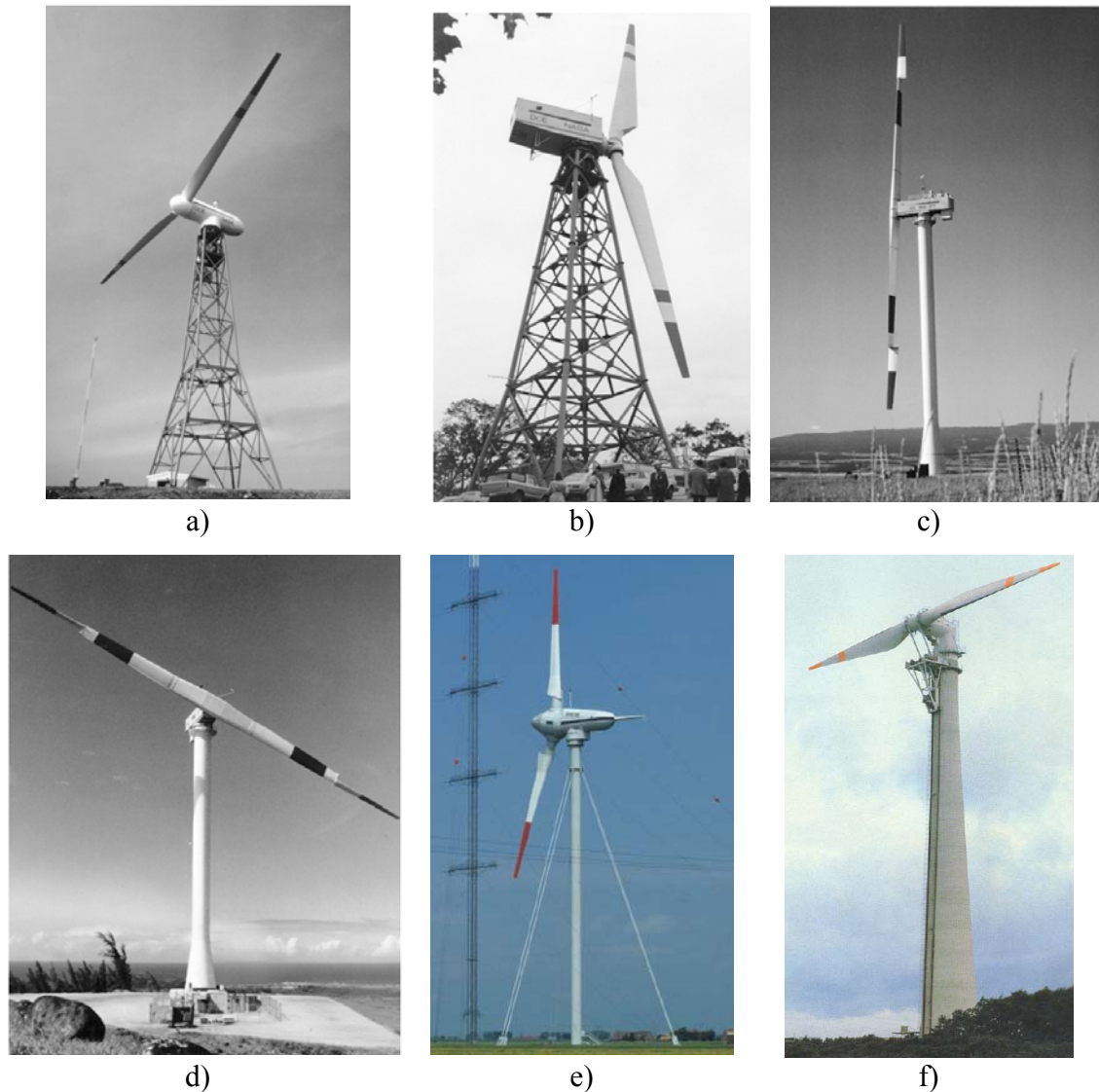
Figure 2.21: Aluminum and steel bladed wind turbines. a) MOD-0 – aluminum blades, b) MOD-1 – steel spar design with foam trailing edge section, c) MOD-2- full steel blade design, d) MOD-5b – full steel blade design, e) GROWIAN – steel spar with GFRP aerodynamic surfaces, f) Nasüdden/WTS-75 - steel spar with GRFP aerodynamic surfaces.
