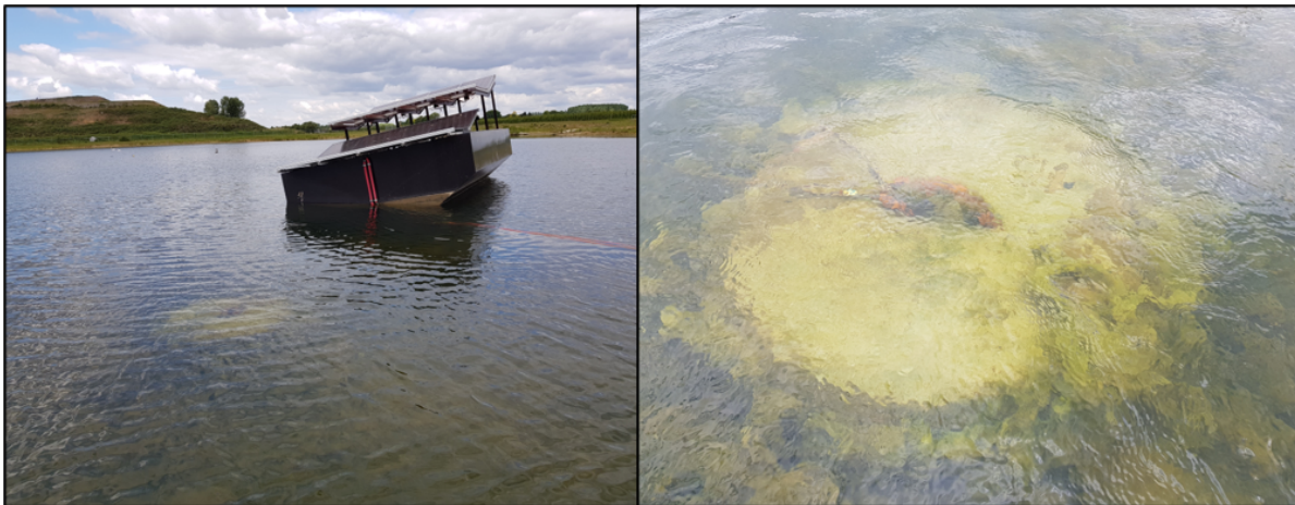
Figure 4.4: The picture on the left shows the Tracker System with in the foreground one of the anchor points. The picture on the right shows a close-up of this anchor point.
