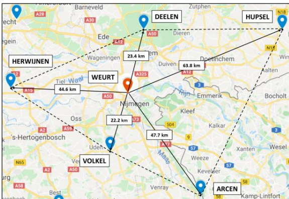
Figure 6. Geographical representation of the five meteorological stations around the target area. Inverse distance weighted (IDW) method which is applicable to geographical areas with uniform morphology (such as the Netherlands) was used to interpolate the irradiance data. IDW method assumes that objects that are close to one another are more similar than the ones that are farther apart.
