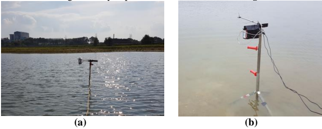
Figure 3. (a) Broadband (285-2800nm), and (b) spectrally-resolved (278-1098nm) albedo measurements at two different spots in the pond.
