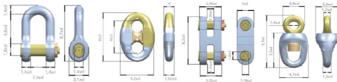
Figure A.7: Shackle (D-type), Kenter, H-type and Swivel connectors. Courtesy: Floating Offshore Wind Farms [7]
