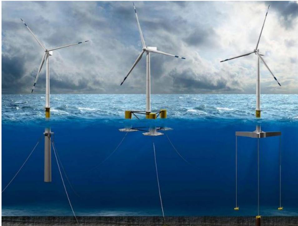
Figure 2.1: Most promising and available floating wind concepts. Courtesy: Floating Offshore Wind Farms [7]
