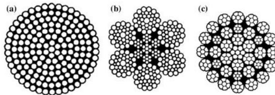
Figure A.6: Spiral strand, six strand and multi-strand cable. Courtesy: Floating Offshore Wind Farms [7]
