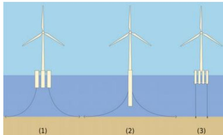
Figure A.1: Floating wind concepts. Courtesy: Floating Offshore Wind Farms [7]
