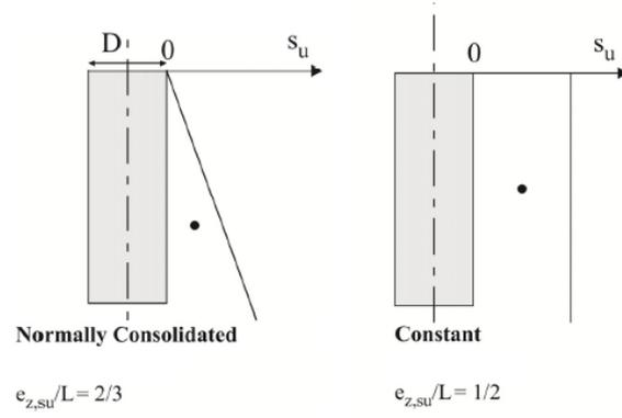
Figure 4.11: Normally consolidated and constant clay layer depiction of the undrained shear strength over the depth. Courtesy: Kay & Palix (2010, 2011, 2015) [22] [23] [30]
