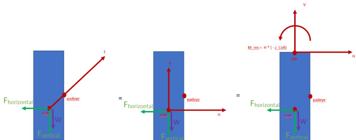
Figure 4.3: Explanation of the load reference point which eliminates the moment in the free body diagram ( $M_{LRP}$ )
