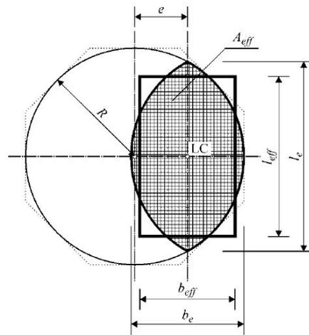
Figure B.1: Effective area of a circular foundation. Courtesy: DNVGL-RP-C212 Offshore Soil Mechanics and Geotechnical Engineering
