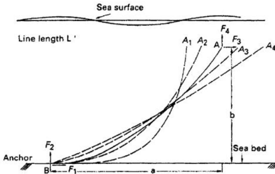
Figure 2.2: Shape of catenary mooring line at different positions. Courtesy: Handbook of Offshore Engineering [8]
