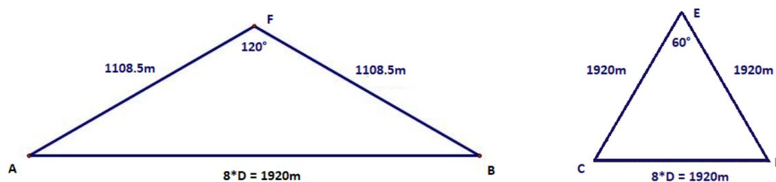
Figure 3.7: Horizontal distances between the centers of rotation of the semi-submersible wind turbines and the center of the suction pile anchor
