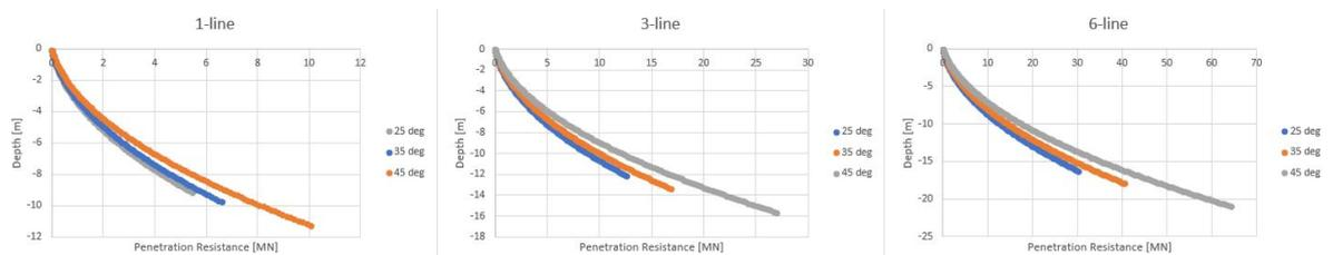
Figure 4.13: Penetration resistance of the sand profile over the depth for different multiline systems
