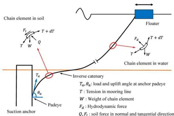
Figure 4.4: Inverse catenary shape due to the connection point beneath the mudline. Courtesy: [36]
