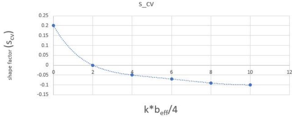
Figure 4.8: Shape factor for circular foundations ( $s_{cv}$ ) taken from DNVGL-RP-C212
