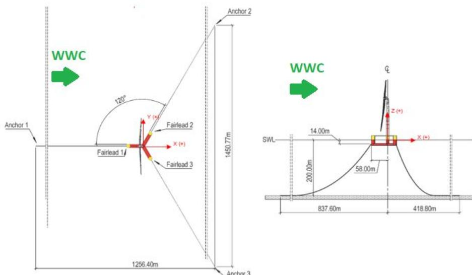
Figure 4.1: Configuration of the original single-line anchoring and mooring set up from the NREL and Umaine 15MW turbine. Courtesy NREL and Umaine [1]
