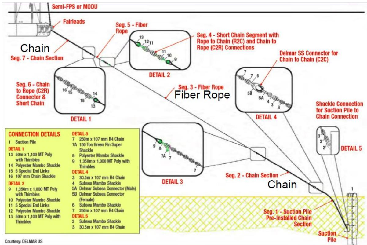
Figure A.4: Example of a combined mooring system for a Semi-FPS or MODU. Courtesy: DELMAR US. Taken from "Floating Structures & Offshore Moorings Mooring Systems - Lecture 12 Mooring Systems" [33].
