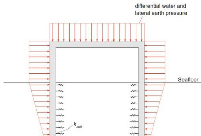
Figure 4.14: Structural integrity assessment of the suction pile anchor installation at an arbitrary situation
