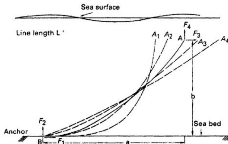
Figure A.2: Shape of catenary mooring line at different positions. Courtesy: Handbook of Offshore Engineering [8]
