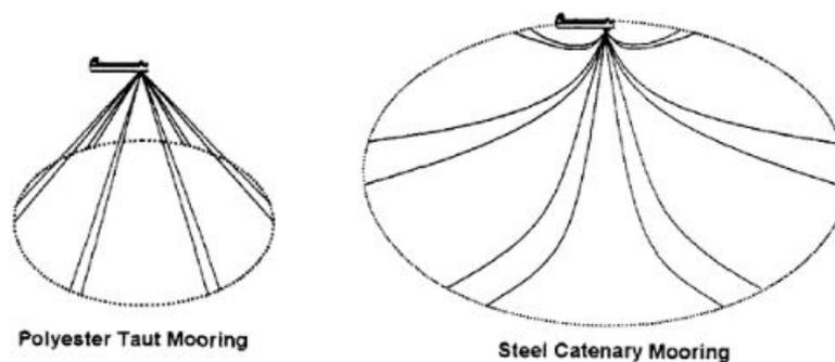
Figure 2.3: Taut system and Catenary system visualised. Courtesy: Handbook of Offshore Engineering [8]
