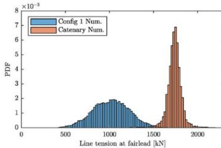
Figure 4.5: Taut vs catenary line tension at fairlead for a 10MW Tetraspar wind turbine at a depth of 180m and a 50-year survival wave condition [3]
