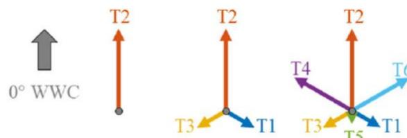
Figure A.15: Multiline vector forces for 1-, 3- and 6-line anchor for 0° wind, wave and current (WWC). Courtesy: Casey Fontana [13]
