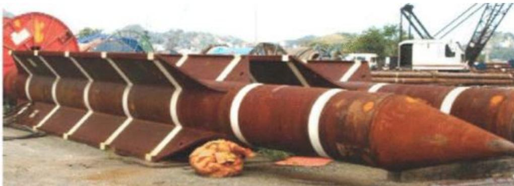
Figure A.11: Torpedo Anchor a gravity installed anchor. Courtesy: InterMoor
