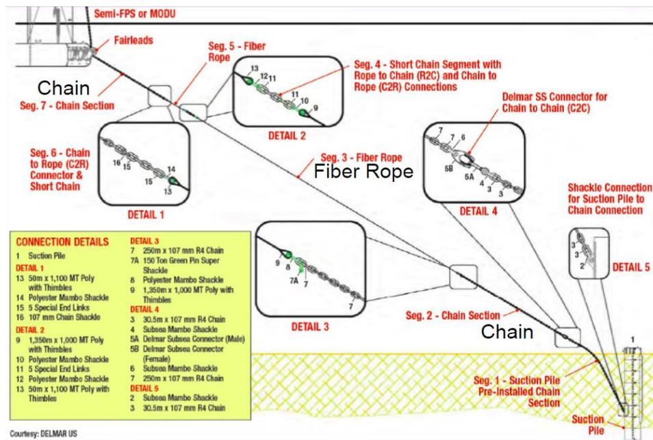
Figure 2.4: Example of a combined mooring system for a Semi-FPS or MODU. Courtesy: DELMAR US. Taken from "Floating Structures & Offshore Moorings Mooring Systems - Lecture 12 Mooring Systems" [33].
