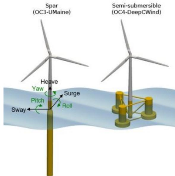
Figure A.17: The NREL 5MW turbine 1) SPAR 2) Semi-submersible. Courtesy: NREL[20]
