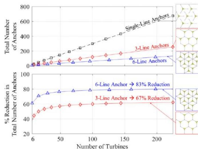
Figure 2.7: Total percentage of the reduction in the amount of anchors needed for a multiline system. Courtesy: Casey Fontana [15]
