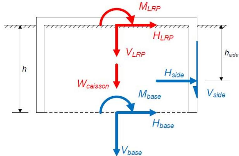
Figure 4.2: Free body diagram of a suction pile
