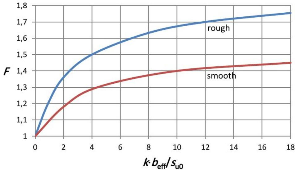
Figure 4.7: Correction factor for rough and smooth footing taken from DNVGL-RP-C212
