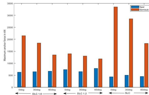
Figure A.18: Maximum anchor tension force in 0°, 30°, 60°WWC for all load cases [4]
