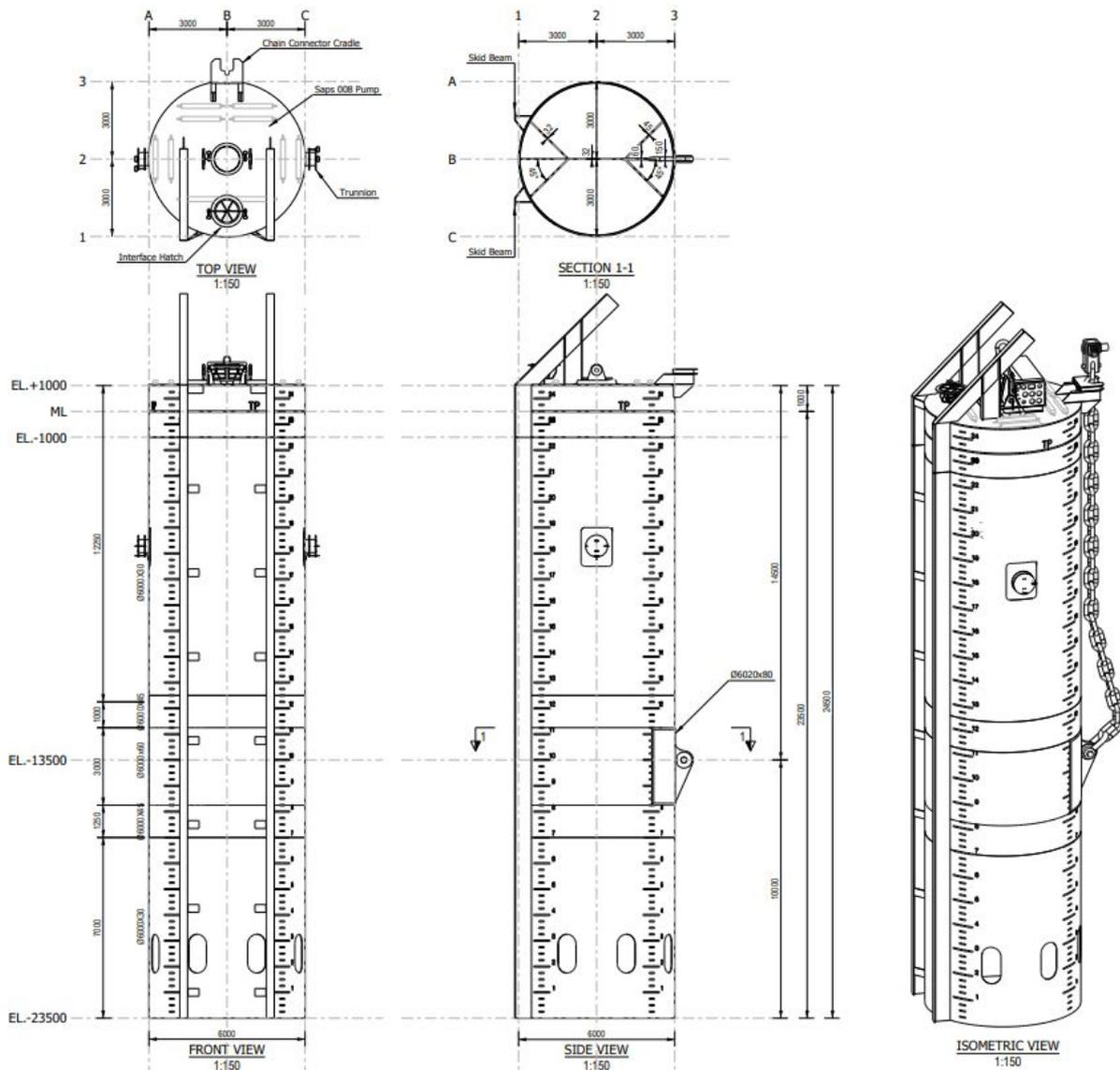
Figure 5.1: Deep water clay suction pile anchor designed for a Floating Production, Storage and Offloading unit
