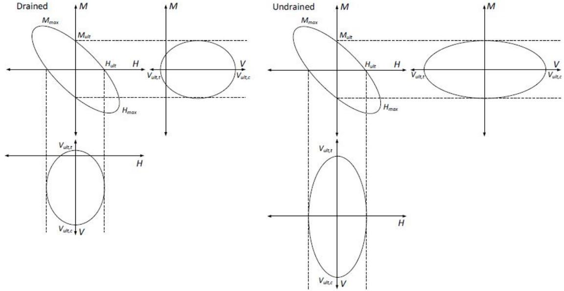
Figure 4.10: VHM failure envelopes for conceptual shallow skirted foundations under drained and undrained loading
