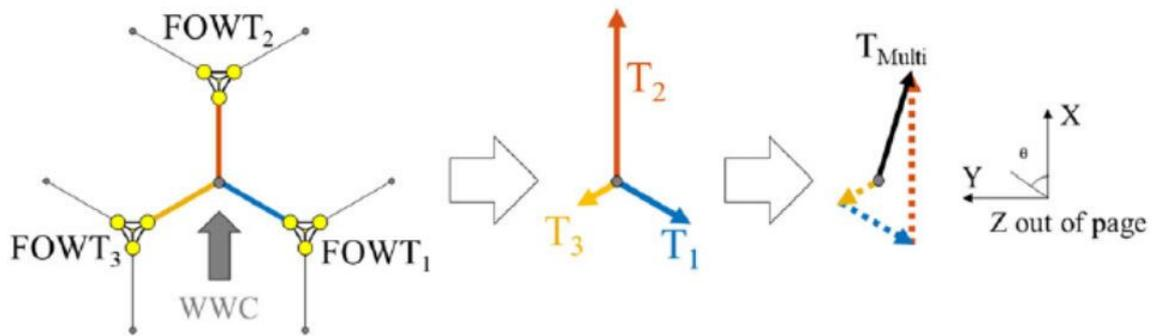
Figure A.14: Multiline net force on a single anchor. Courtesy: Casey Fontana [13]
