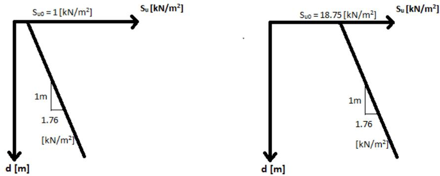
Figure 4.6: Shear strength profile of the two clay profiles: 1) normally consolidated clay 2) slightly overconsolidated clay
