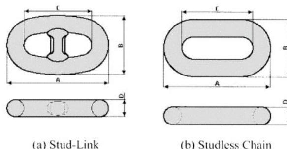
Figure A.5: Stud-link chain vs Studless chain. Courtesy: Handbook of Offshore Engineering [8]
