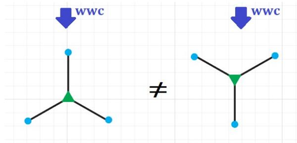
Figure 3.5: Two different situations for the semi-submersible anchor system
