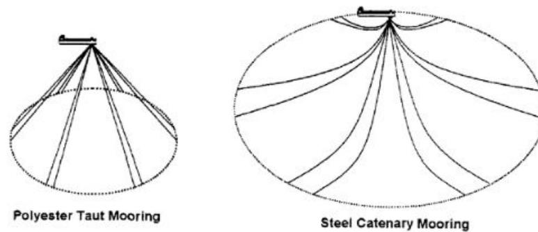
Figure A.3: Taut vs Catenary system. Courtesy: Handbook of Offshore Engineering [8]
