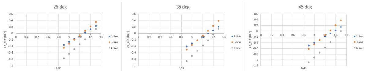
Figure 4.15: Maximum suction minus the critical piping suction for different embedment ratios
