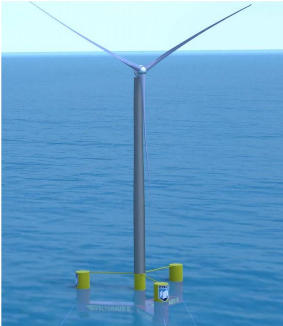
Figure 3.1: A picture showing the university of Maine reference platform designed to support the IEA-15-240 RWT system definition. Courtesy: University of Maine [1]
