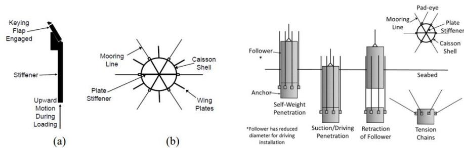
Figure A.20: Overview of an MRA and strategies for enhancing load capacity of MRA with a) keying flaps and b) wing plates and the installation procedure of an MRA using a suction pile. Courtesy J. Lee [24]
