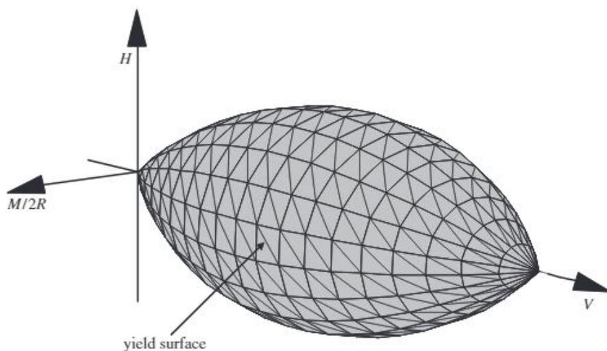
Figure 4.9: Conceptual 3D depiction of a VHM-envelope/yield of a flat footing on sand. Courtesy: Byrne (2004) [6]
