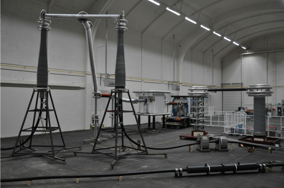
Figure 3.1: Set up for the DC test performed at the DNV GL HV laboratories
