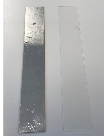
Figure 6.15: Aluminum tape stuck to a strip
