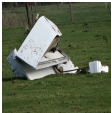
(b) Torn parts of the antenna
