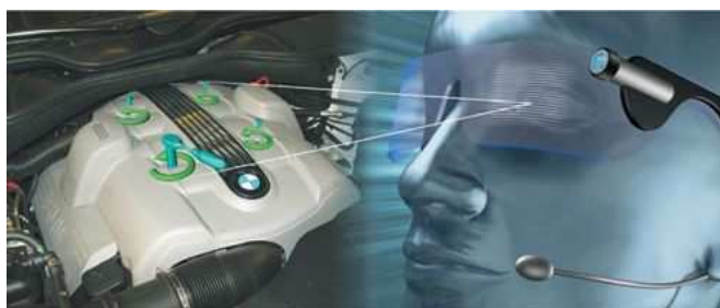
Figure 1-9 An AR system proposed by BMW for an innovative repair manual [7]. Left: The real engine, superimposed with a virtual screwdriver and an arrow that shows the direction in which the user must turn. Right: impression of future AR glasses.
