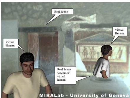
Figure 1-7 Immersive video see-through application. Output of the lifePLUS project [4] with animated characters at the historical site of Pompeii. This system uses camera images to track the position of the user and requires off-line learning of the environment as no special objects are added to the scene for tracking (markerless tracking).
