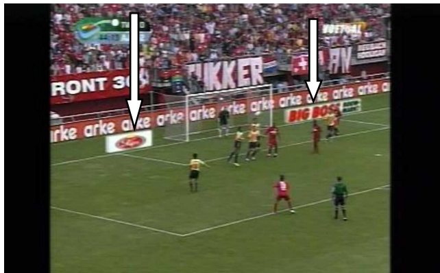
Figure 1-3 Example of Real-time-AR. Virtual advertising boards are projected at the sides of the goal. The camera’s pan, tilt and zoom information is extracted from the images and used to correctly display the virtual environment. (ADVision from Orad: www.orad.tv )
