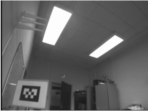
Figure 3-42 Example picture taken by our JAI camera mounted on a pan-tilt unit. The camera was panned to the right by 30° and tilted backwards by 30°. The marker had a fixed pan of 30°.
