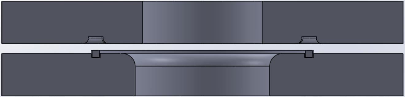
Figure 4.2: The drawbead design in the upper and lower die shown in Solidworks.
