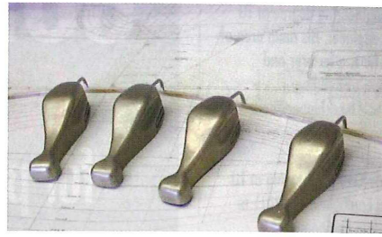
Fig. 5: Splines used e.g. for ship design
