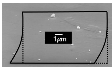
Figure 3.17: Drift of the electron beam.
