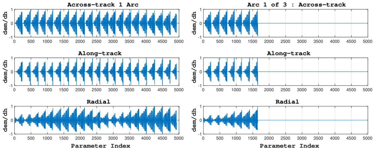
(a) This figure illustrates the partials for a single arc of 3.5 months. (b) This figure illustrates the partials for arc 1 of 3 arcs.
