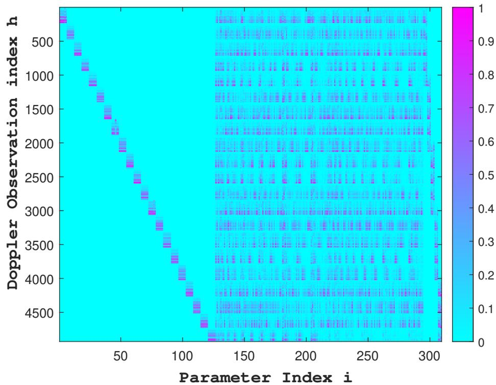
Figure B.22: This figure illustrates the H matrix for empirical accelerations of 5 arcs. The H matrix contains partial derivatives, representing uncertainty in Doppler observations w.r.t uncertainty in parameters ( $\frac{\partial h}{\partial i}$ ). The vertical axis represents the total number of Doppler observations generated. The parameters on the horizontal axis represent the states (1 to 126), the gravity field coefficients (127-294) and the empirical accelerations (295-309).
