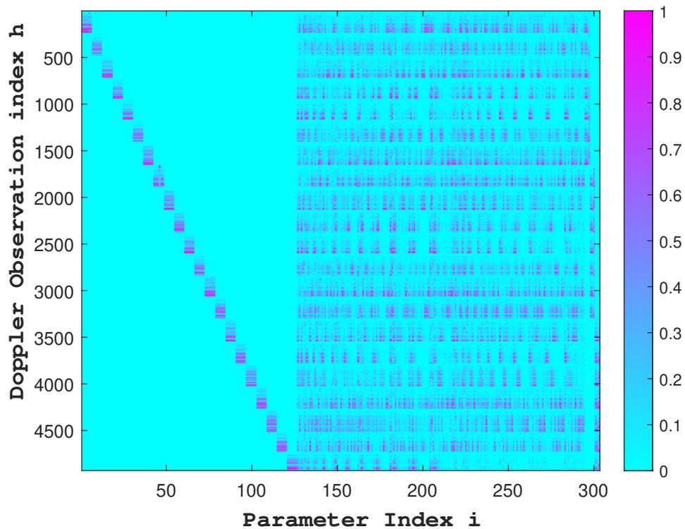
Figure B.21: This figure illustrates the H matrix for empirical accelerations of 3 arc. The H matrix contains partial derivatives, representing uncertainty in Doppler observations w.r.t uncertainty in parameters ( $\frac{\partial h}{\partial i}$ ). The vertical axis represents the total number of Doppler observations generated. The parameters on the horizontal axis represent the states (1 to 126), the gravity field coefficients (127-294) and the empirical accelerations (295-303).
