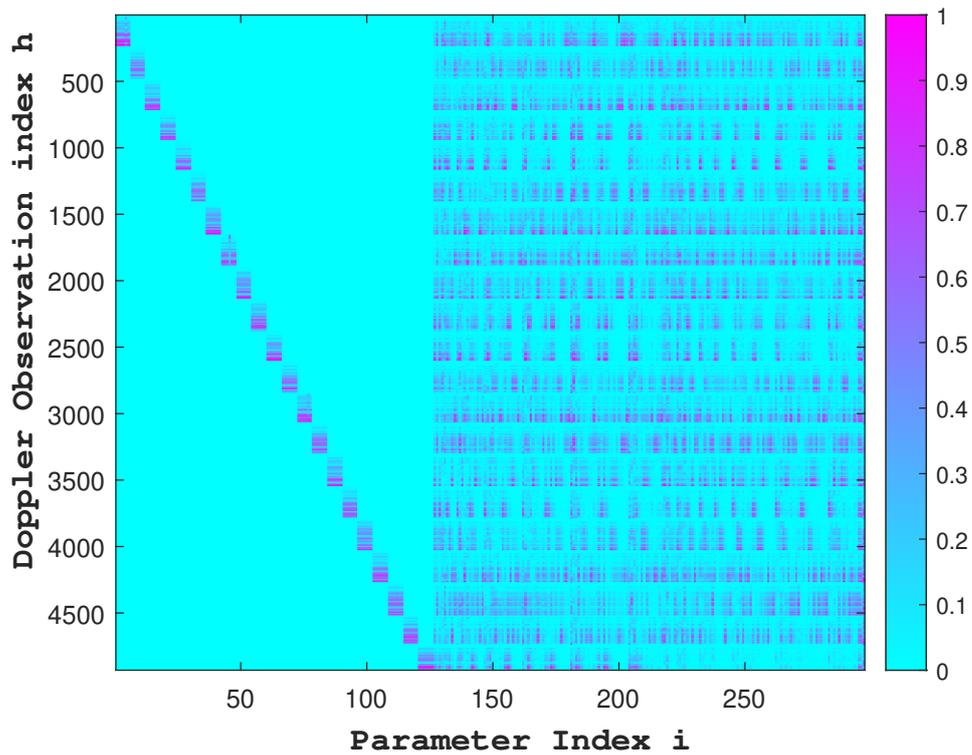
Figure B.20: This figure illustrates the H matrix for empirical accelerations of 1 arc. The H matrix contains partial derivatives, representing uncertainty in Doppler observations w.r.t uncertainty in parameters ( $\frac{\partial h}{\partial i}$ ). The vertical axis represents the total number of Doppler observations generated. The parameters on the horizontal axis represent the states (1 to 126), the gravity field coefficients (127-294) and the empirical accelerations (295-297).
