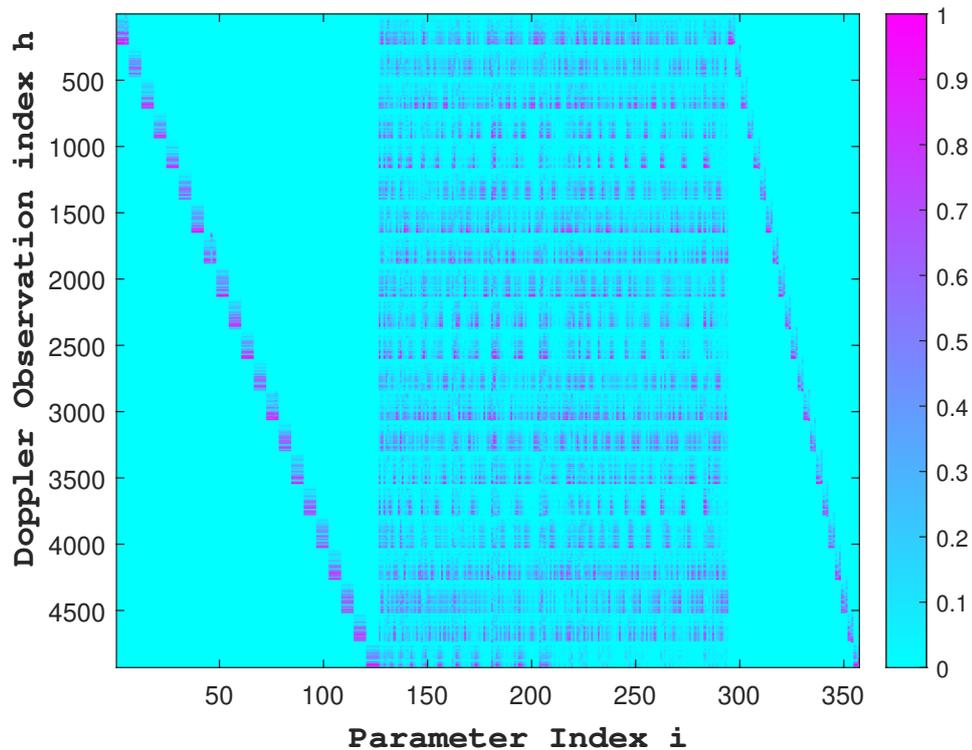
Figure B.23: This figure illustrates the H matrix for empirical accelerations of 21 arcs. The H matrix contains partial derivatives, representing uncertainty in Doppler observations w.r.t uncertainty in parameters ( $\frac{\partial h}{\partial i}$ ). The vertical axis represents the total number of Doppler observations generated. The parameters on the horizontal axis represent the states (1 to 126), the gravity field coefficients (127-294) and the empirical accelerations (295-357).
