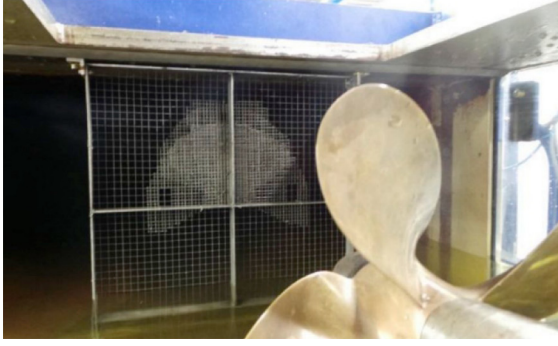
(a) Propeller behind a wake screen (Aktas, 2017).
